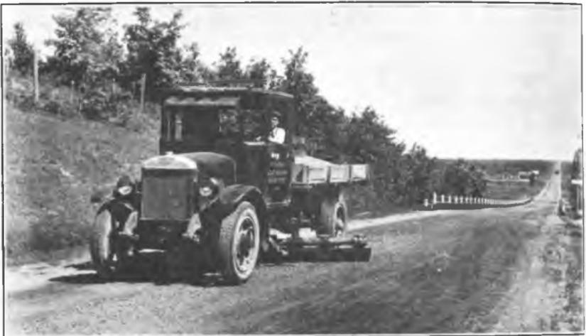
Fig. 1. Spring Blade attached to truck.
