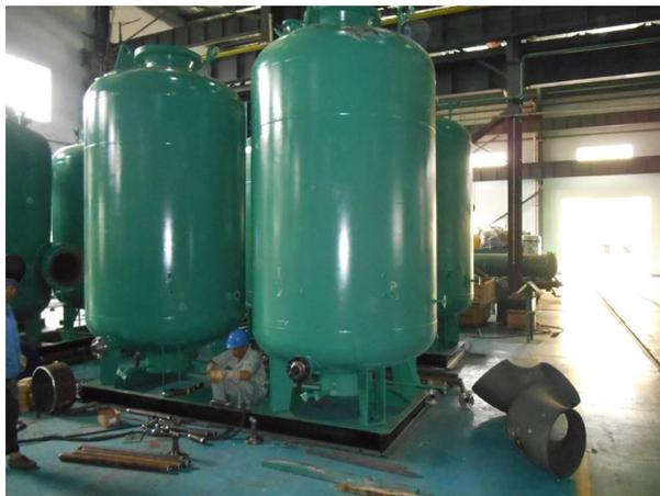
Figure 6: Oil Separator Skid
