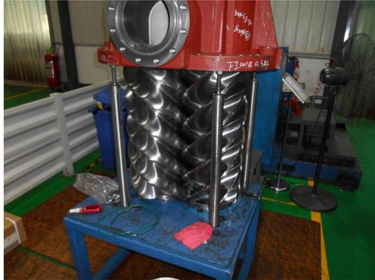
Figure 1 Screw expander assembly
