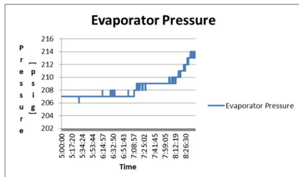
Figure 13: Ramp Up Effect on Evaporator Pressure
