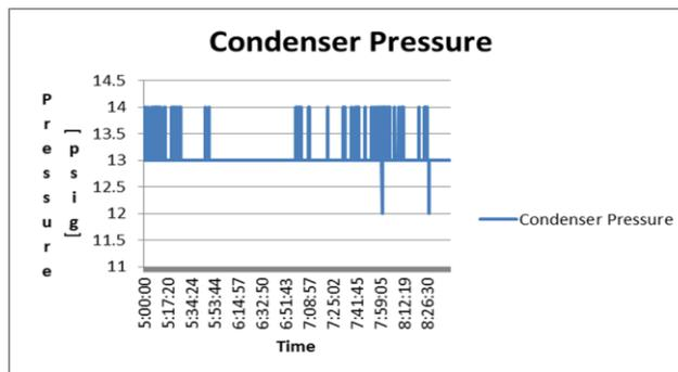
Figure 14: Ramp Up Effect on Condenser Pressure
