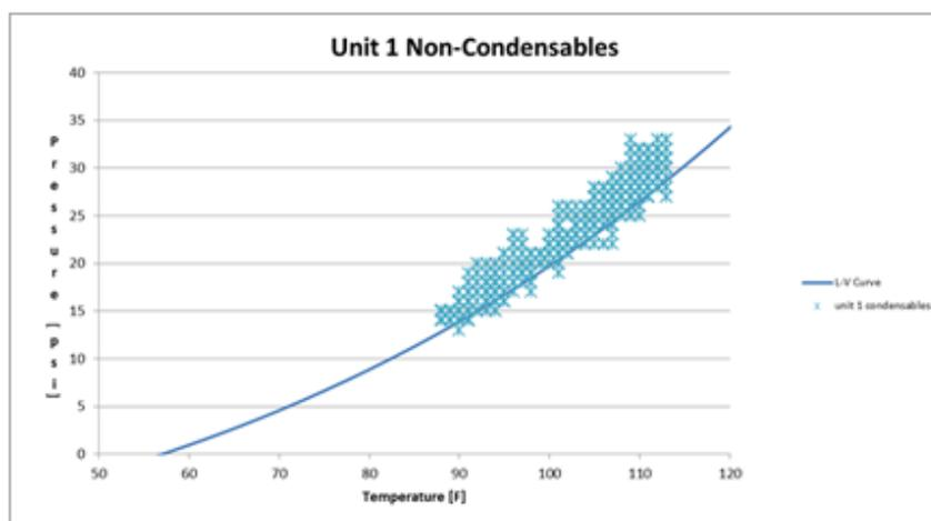
Figure 16: Unit Condenser Curve After Purging
