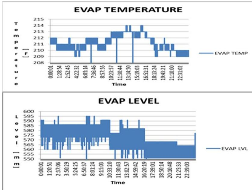
Figure 11: Evaporator Temperature Change with Evaporator Level
