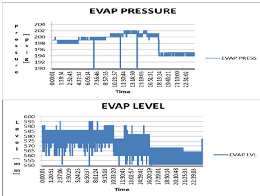
Figure 10: Evaporator Pressure Change with Evaporator Level
