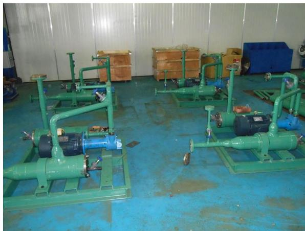
Figure 7: Oil Pump Module Assembly
