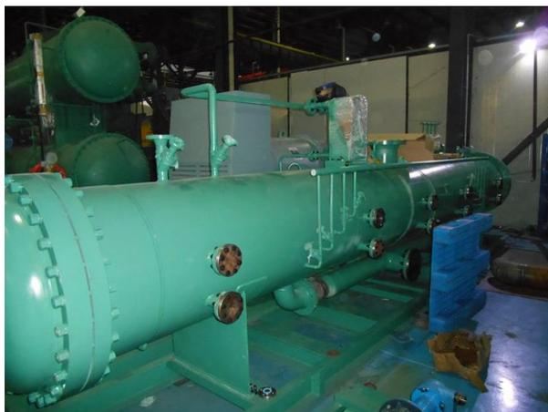
Figure 4: Evaporator Module Assembly
