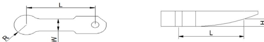
**Figure 4:** Shape of the stopper used in the experiment
