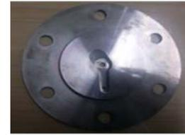
**Figure 3:** The orifice plate1
