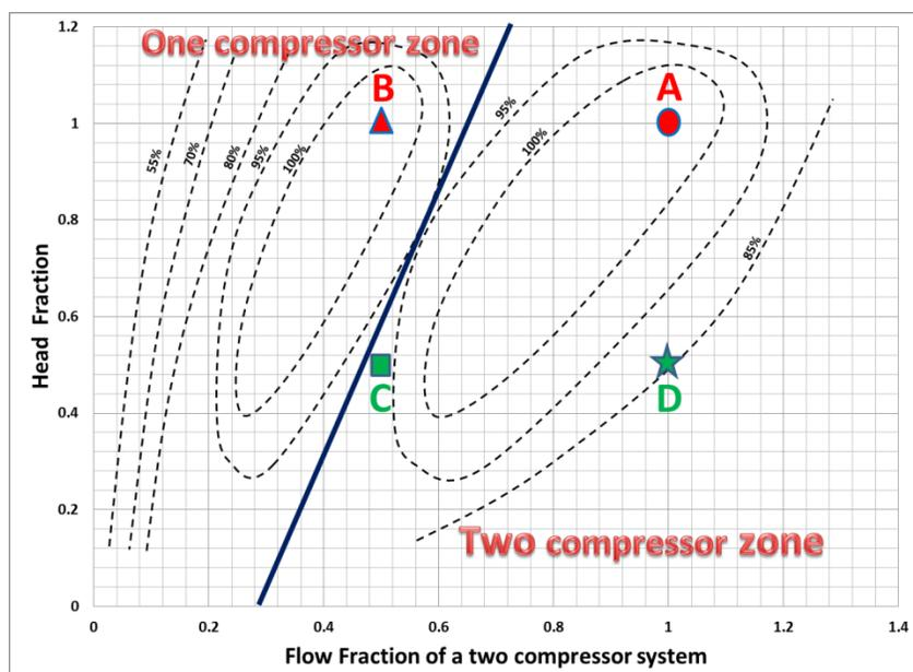
**Figure 3:** Aerodynamic efficiency islands of a two-compressor system
