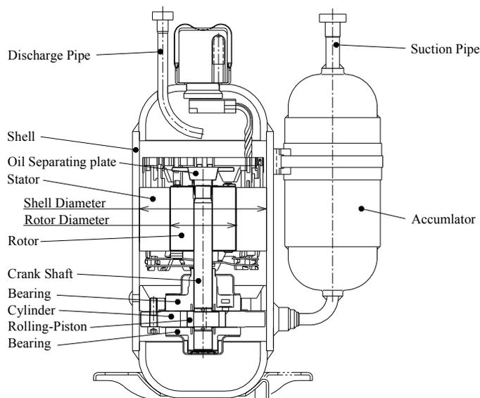
**Figure 1:** CO<sub>2</sub> rotary compressor
