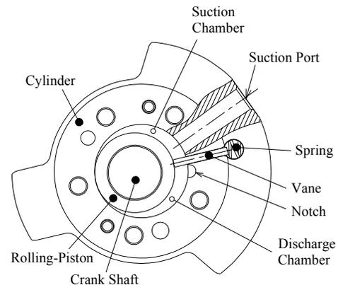
**Figure 2:** Compression Mechanism
