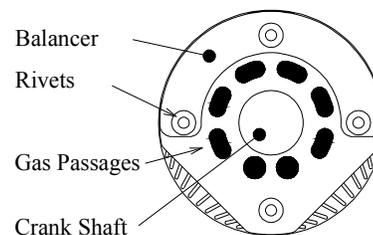
**Figure 3:** Motor rotor
