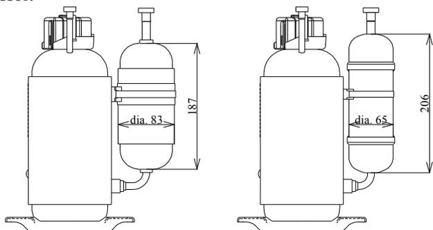
Compressor with Original Accumulator Compressor with Improved Accumulator
