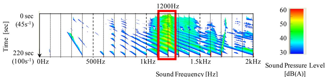
**Figure 12:** The result of run-up test (from  $45\text{s}^{-1}$  to  $100\text{s}^{-1}$ )
