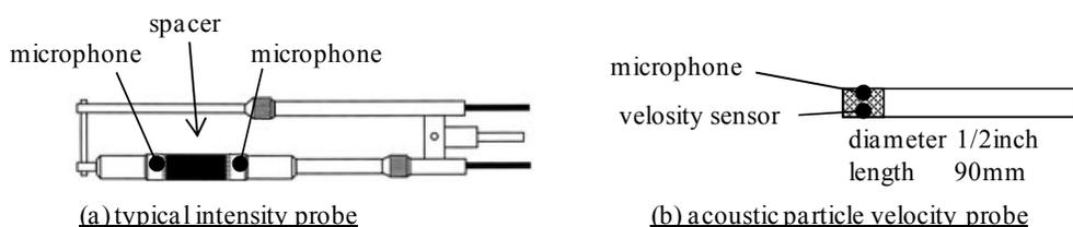
(a) typical intensity probe (b) acoustic particle velocity probe
