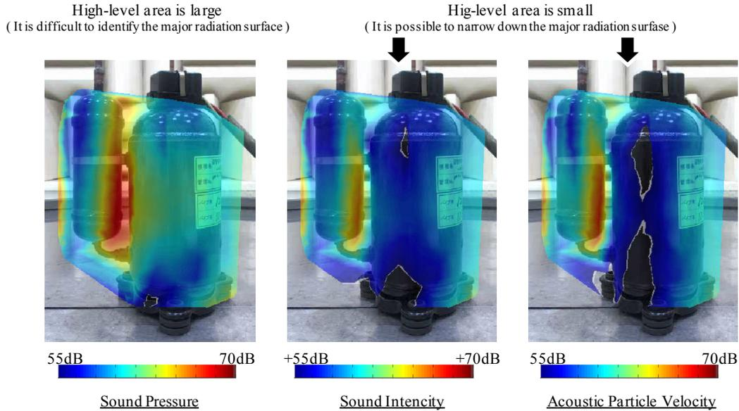
**Figure 18:** Sound maps of improved compressor, 1.6-kHz band
