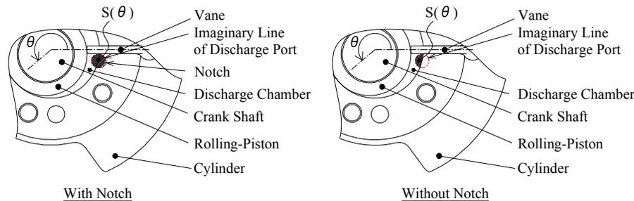
**Figure 4:** Cross-Sectional Area of outlet of Discharge Chamber
