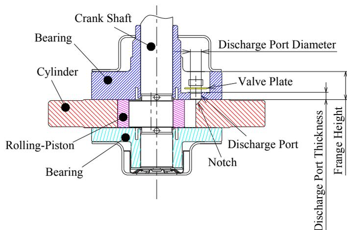
**Figure 6:** Cross section of compression Mechanism
