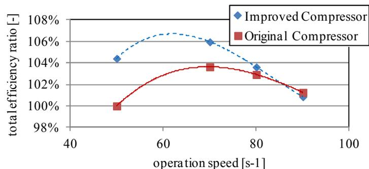
**Figure 11:** Relationship between operation speed and total efficiency ratio
