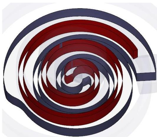
**Figure 1:** A typical CAD surfaces input by user, stationary rotor in grey, orbiting rotor in red.
