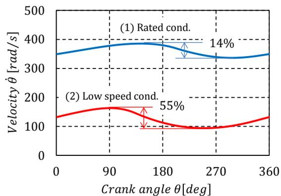
Figure 11: Angular velocity of crankshaft
