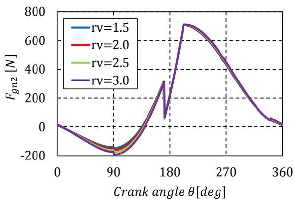
Figure 13: Contact force  $F_{gn2}$  between vane and cylinder
