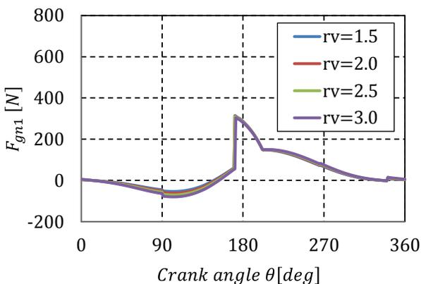
Figure 12: Contact force  $F_{gn1}$  between vane and cylinder
