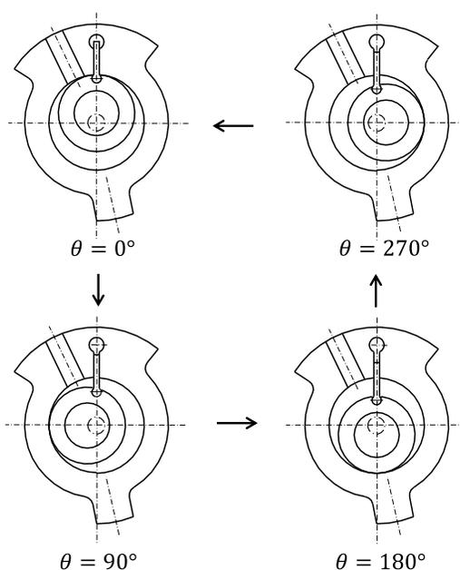
**Figure 1:** Compression process of new rotary compressor
