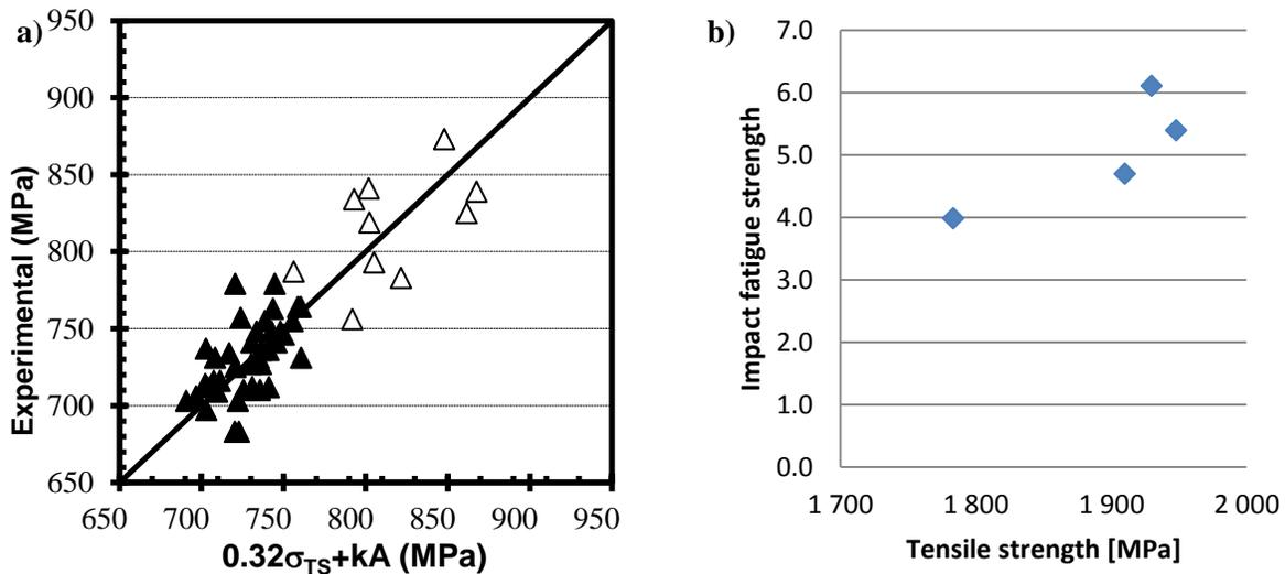
**Figure 6:** (a). Bending fatigue strength of the flapper valve steel strips versus tensile strength  $\sigma_{TS}$  and ductility/elongation A (k is the constant between 18.8 to 25.1 depending on the material) (b). Impact fatigue strength versus tensile strength for the modified AISI 420 type of flapper valve strip.
