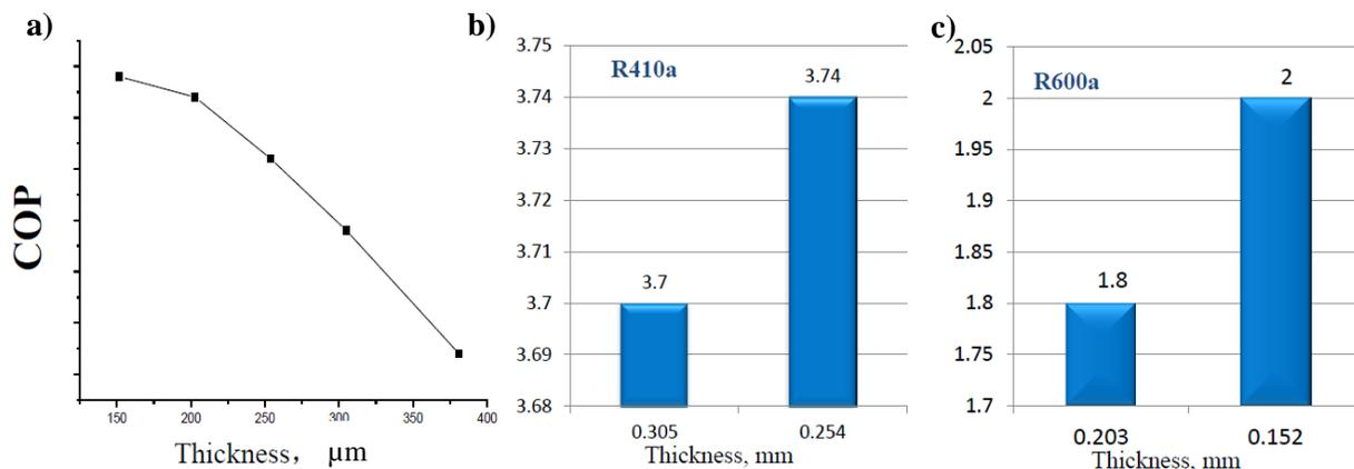
**Figure 9:** In a) an overview of COP as a function of valve thickness is shown. In b) and c) the specific difference in COP as the valve thickness is reduced for the different media R410a and R600a, respectively.
