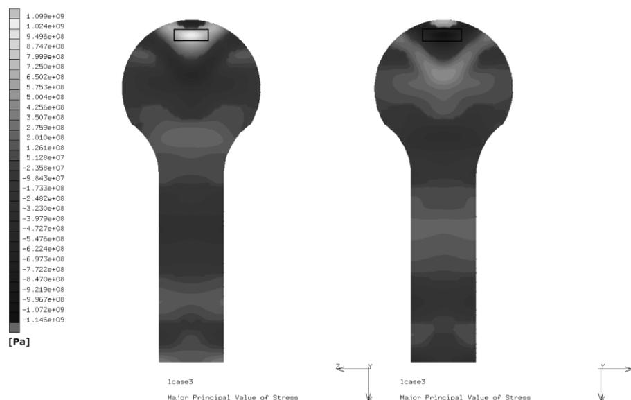
**Figure 1:** The left and right picture shows the top and bottom of the flapper valve, respectively. Both pictures were taken at a time where the maximum tensile – and compressive stresses occurred. The figures are from a 80 Hz case.
