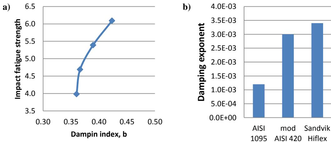
**Figure 7:** a) Influence of damping capacity and material on the impact fatigue strength of the flapper valve strips. b) Damping exponent for the different material AISI 1095, modified AISI 420 and Sandvik Hiflex™
