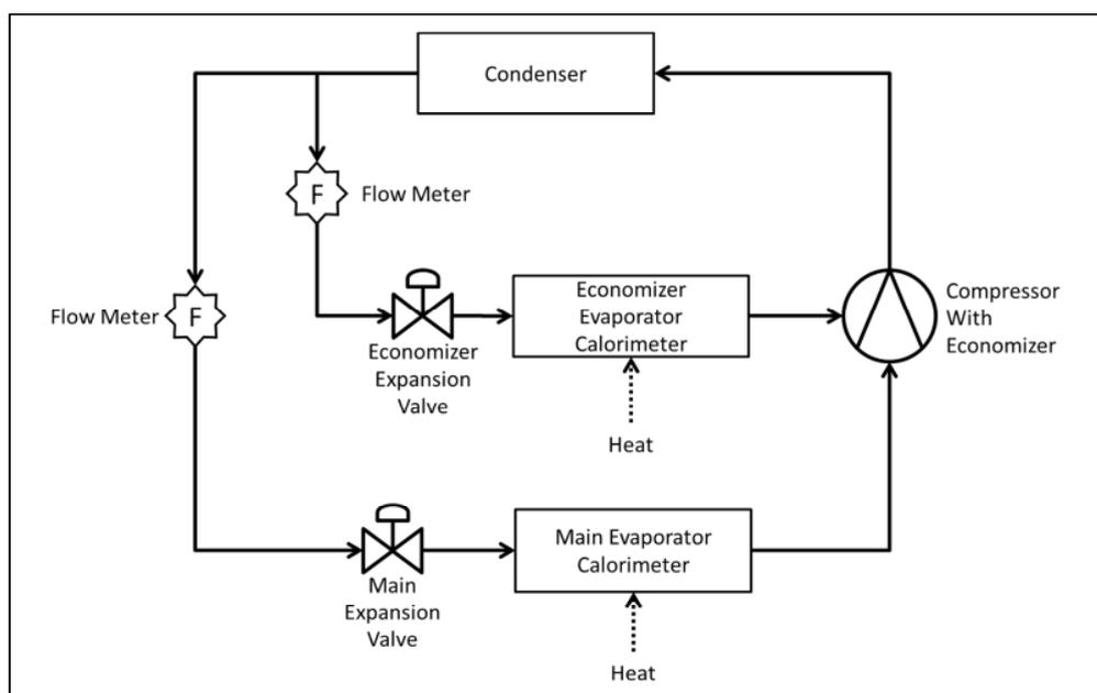
**Figure 3: Test Stand Configuration for Economizer Compressors**
