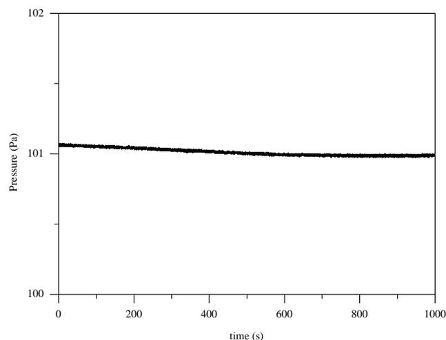
Figure 5: Leak test
