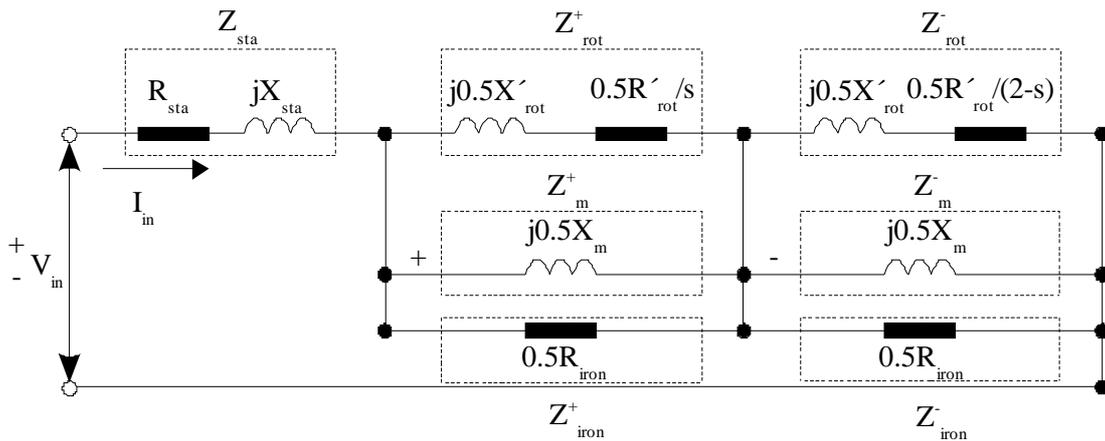
**Figure 2:** Equivalent circuit of a single-phase induction motor.
