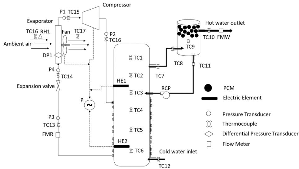
Figure 1: System diagram of HTHP with PCM thermal energy storage
