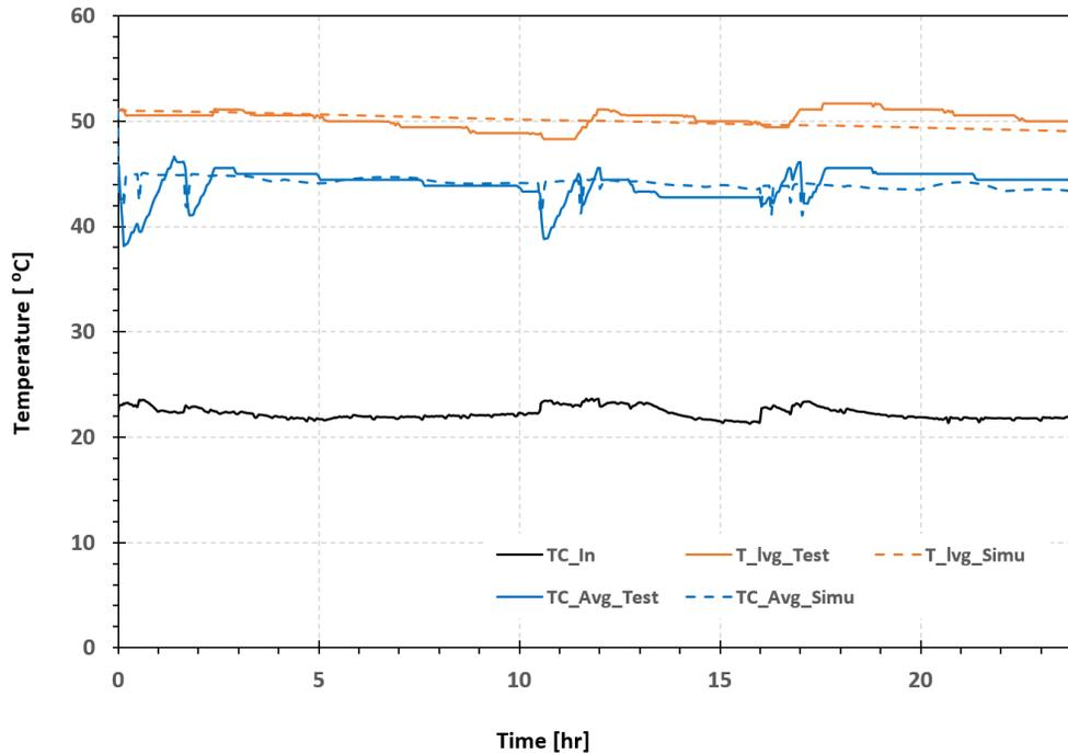
Figure 6. Leaving tank and average tank water temperature: test vs. simulation
