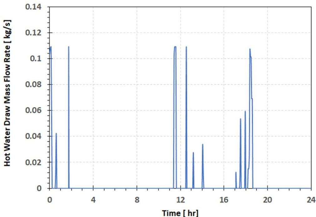
Figure 5. Heat pump water heater draw schedule
