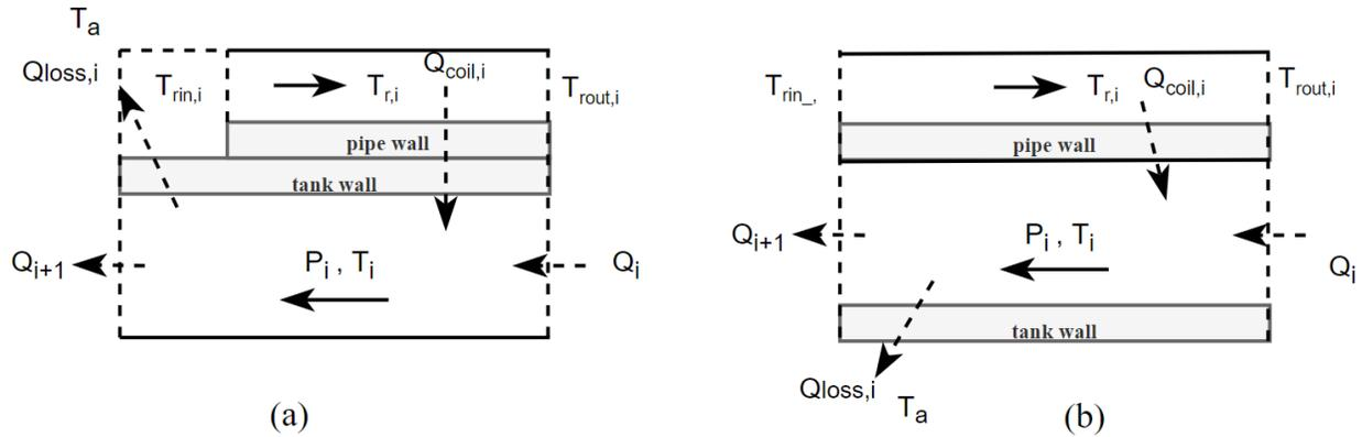
Figure 2: Control volume schematics of (a) wrapped around coil based water tank and (b) immersed coil based water tank.
