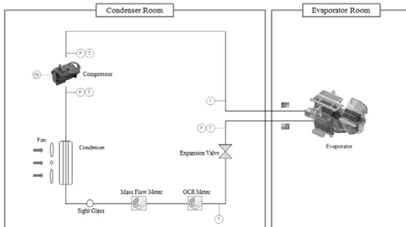
Figure 6 : Schematic diagram of system bench
