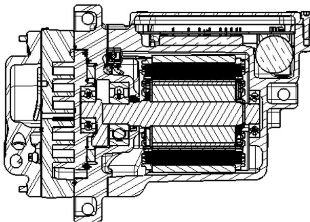
**Figure 1 :** Section view of electrically driven scroll compressor
