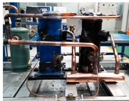
**Figure 2:** Oil return to common suction test
