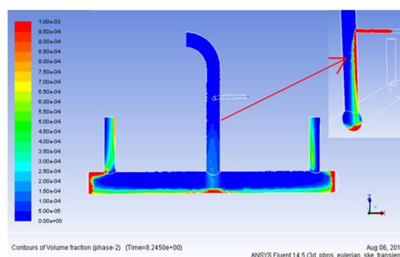
Figure 6: Oil return simulation result
