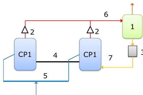
Figure 9: Schematic of oil return to compressor
