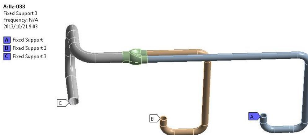
**Figure 12:** discharge pipe model for the first round FEA
