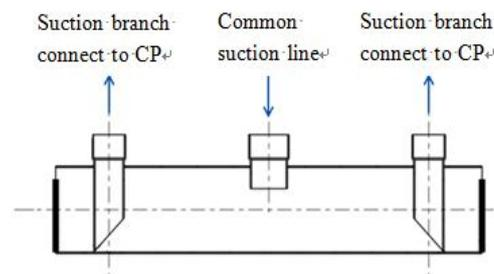
**Figure 4:** Cross-section of suction header
