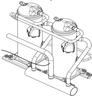
**Figure 3:** Even tandem pipework design
