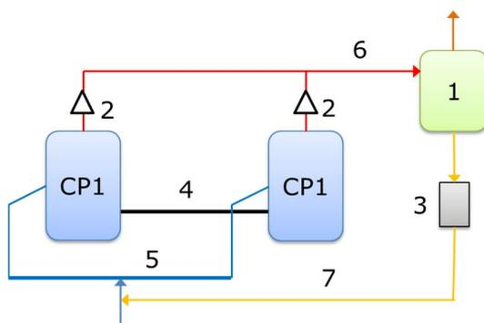
**Figure 1:** Schematic of oil return to common suction
