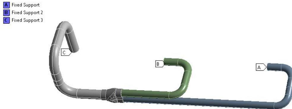
**Figure 14:** discharge pipe model for the third round FEA
