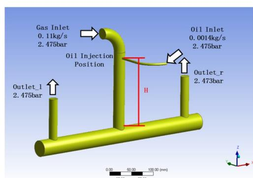
Figure 5: Oil return simulation model
