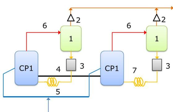
**Figure 10:** Schematic of individual oil return
