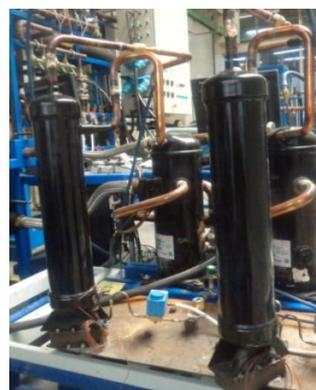
**Figure 11:** Individual oil return test
