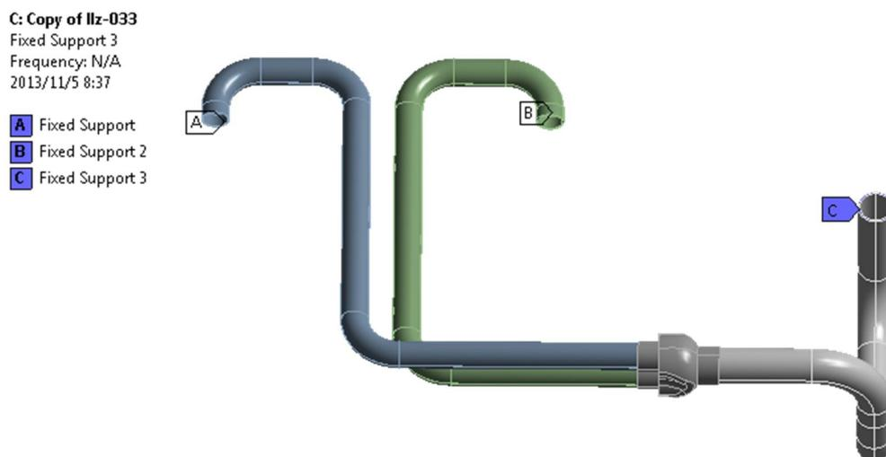
**Figure 13:** discharge pipe model for the second round FEA**Table 7:** Test result for the second round of study
