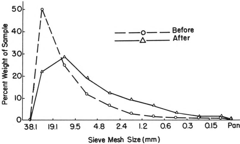
Figure 3. Aggregate Size Distributions for New Providence Shale
