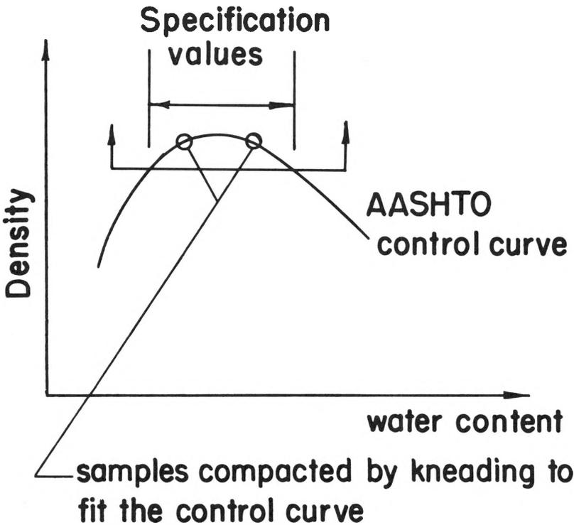
Figure 6. Laboratory Preparation of Strength and Compressibility Samples
