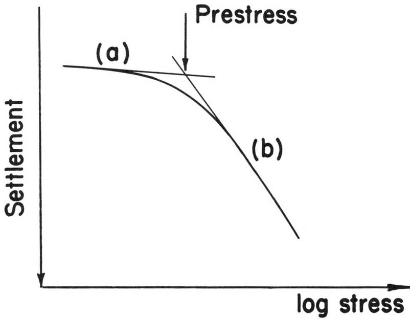
Figure 7. Prestress Established by Rolling
