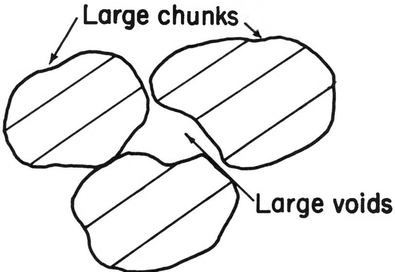
Figure 1. Non Durable Chunks Break Down (Slake) and Fall into Voids
