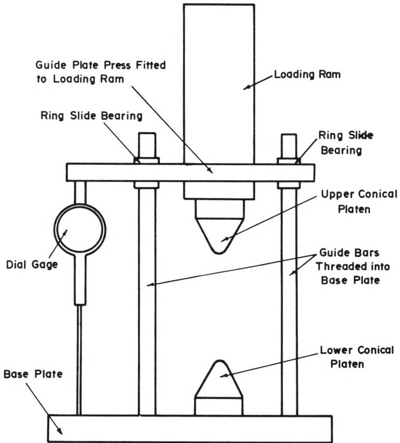
Figure 2. Diagram of Point Load Strength Test Apparatus
