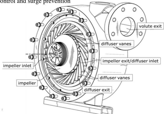
**Figure 8:** Compressor main housing with volute showing the 1<sup>st</sup> stage impeller and vaned diffuser array
