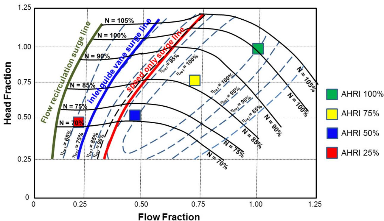
**Figure 12:** Two-stage compressor map showing the difference in stable operating range when using variable speed only, variable speed with inlet guide vanes, and variable speed with inter-stage flow recirculation as control mechanism and the location of the AHRI IPLV test points
