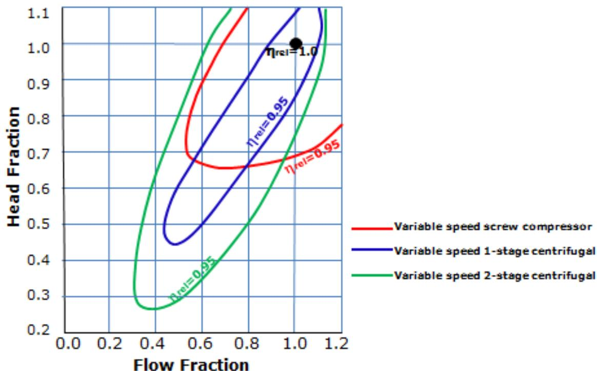
**Figure 1:** The 95% relative efficiency islands on the performance map for three compressor concepts
