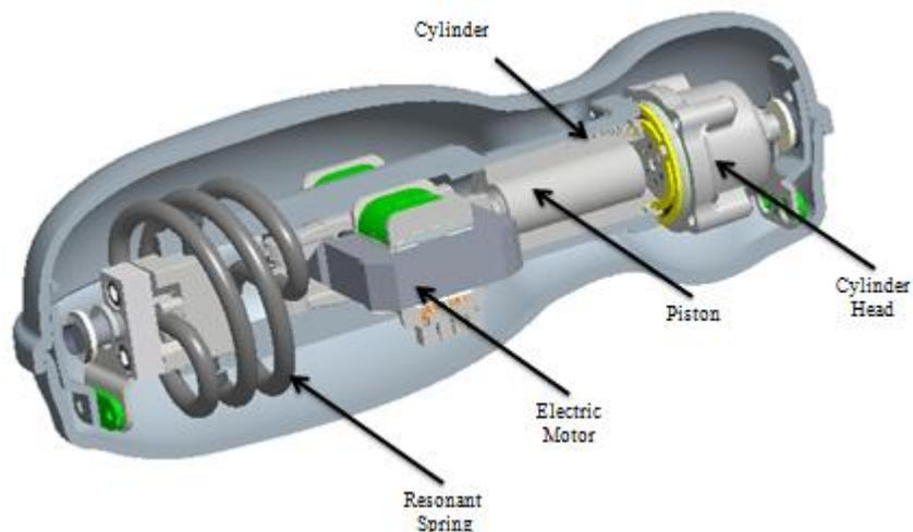
**Figure 2** - Variable capacity linear motor driven scheme.
