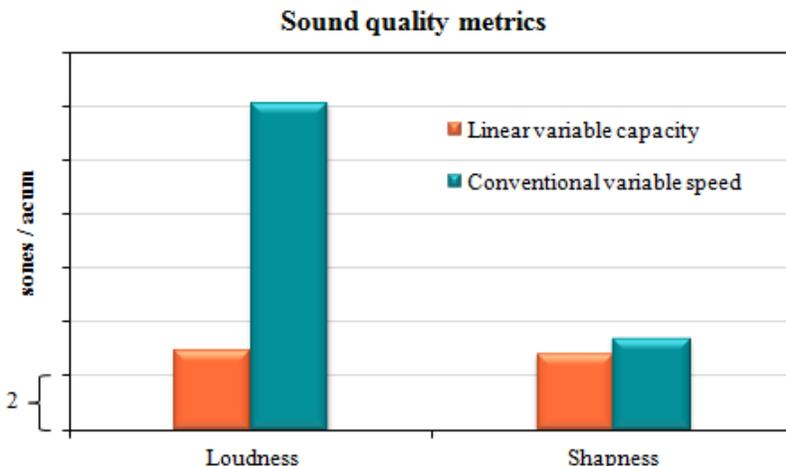
Figure 6 - Sound quality metrics for compressor starting.
