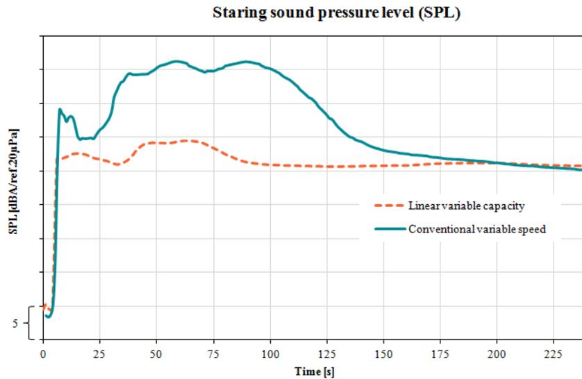
**Figure 4** - Starting sound pressure level comparison.
