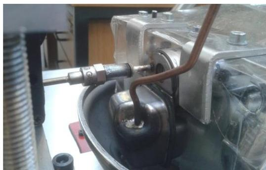
**Figure 5:** Pressure sensor mounted on the valve plate
