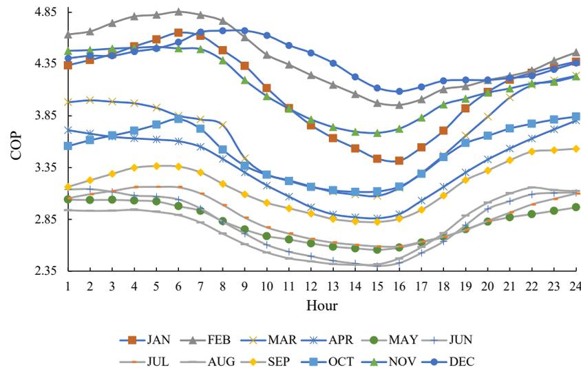
**Figure 3: Cooling coefficient of performance (COP) using the vapor injection (VI) system during 24 hours of the 21st of every month for Kuwait weather.**
