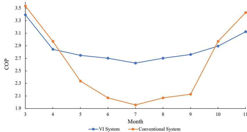
**Figure 2: Results comparison of vapor injection (VI) and conventional vapor compression cycle (VCC) system for monthly cooling coefficient of performance (COP) using the developed empirical equations for Kuwait weather.**
