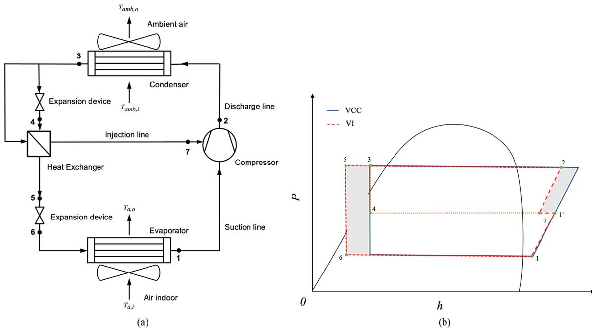
**Figure 1: (a) Schematic of typical cooling cycle setup with vapor injection (VI) configuration, and the corresponding (b) pressure-enthalpy diagram of the VI system compared to the conventional vapor compression cycle (VCC) system.**
