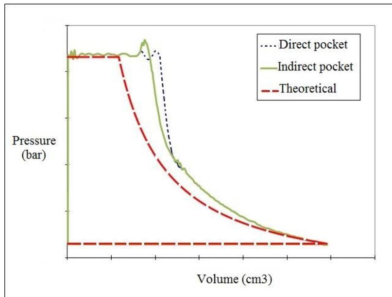
**Figure 8:** Pressure-volume diagram at high pressure ratio
