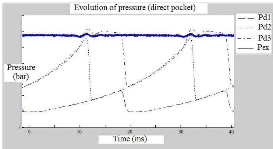
**Figure 4:** Distribution of pressure in the direct pocket
