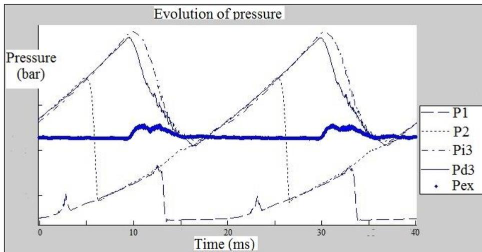
**Figure 11:** Distribution of pressure without IDVs
