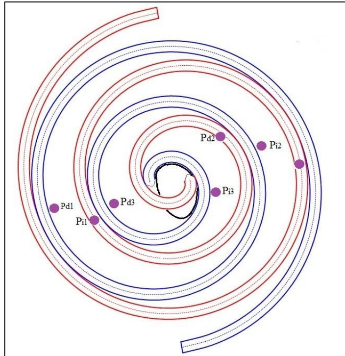
**Figure 1:** Location of the pressure sensors inside the scrolls
