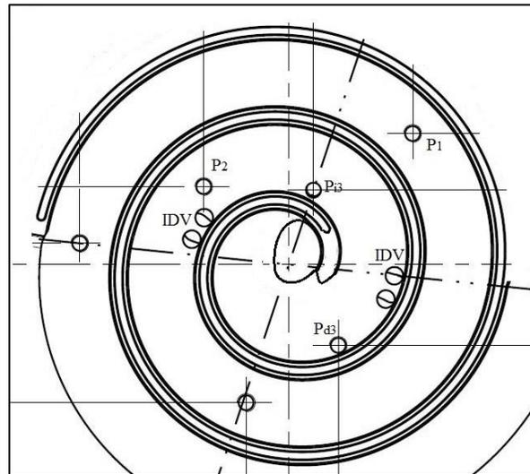
**Figure 9:** Location of the IDVs and of the pressure sensors
