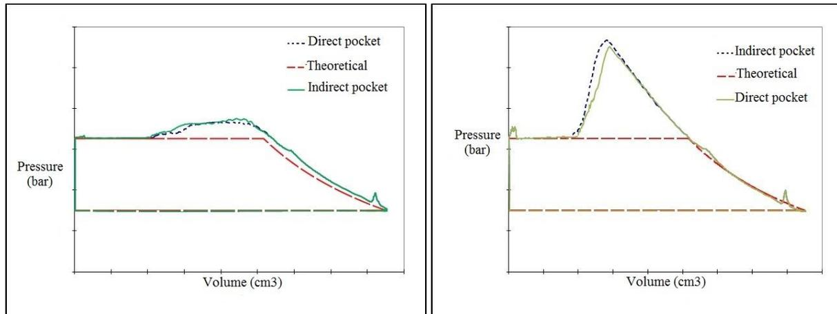
**Figure 12:** Compared pressure-volume diagrams with and without IDV
