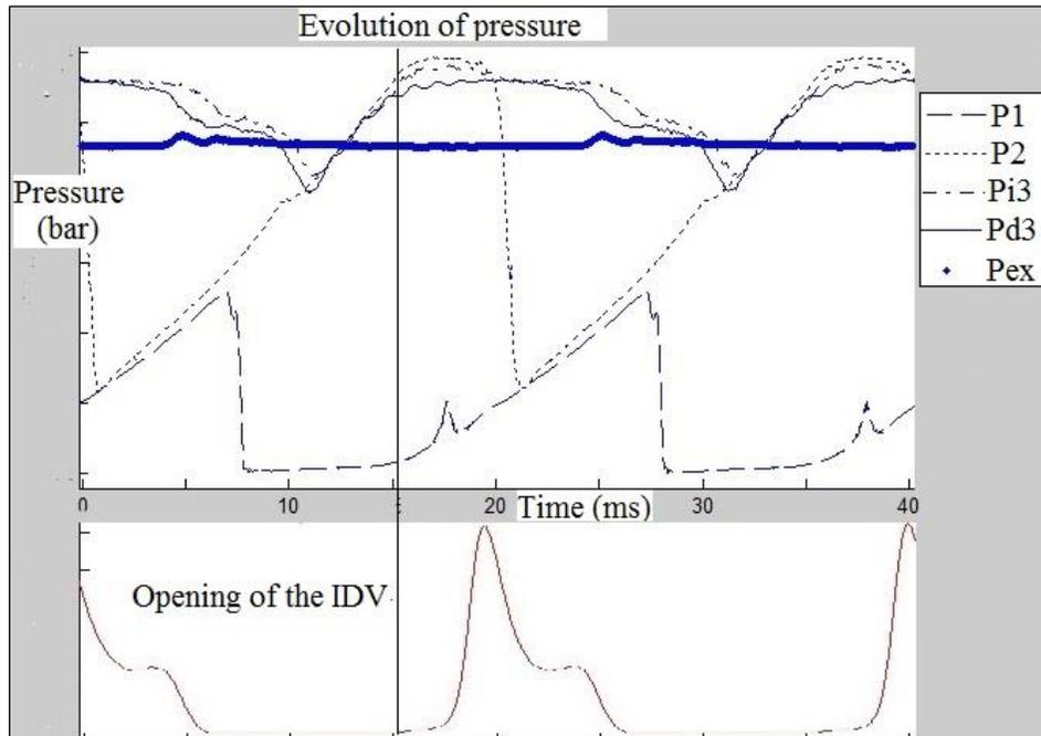
**Figure 10:** Distribution of pressure with IDVs working
