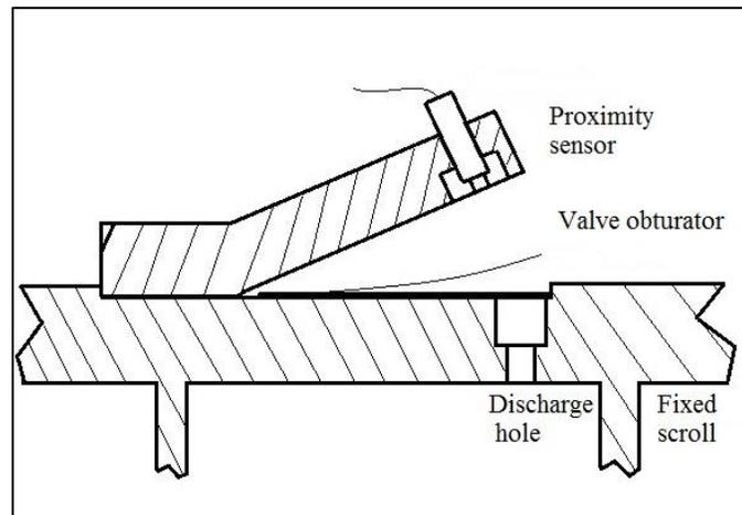
**Figure 3:** Instrumentation of an IDV
