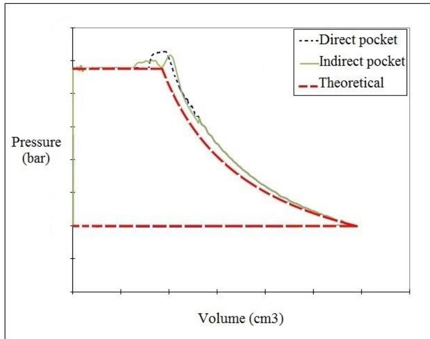
**Figure 6:** Experimental and ideal Pressure-Volume diagrams of the compressor
