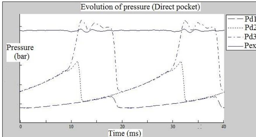
**Figure 7:** High pressure-ratio - pressure in the direct pocket
