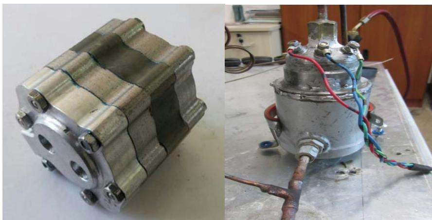
**Figure 6:** New generation Wankel compressor prototype
