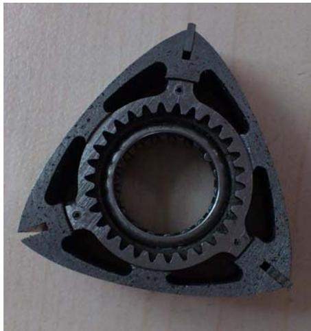
**Figure 7:** Triangular rotor
