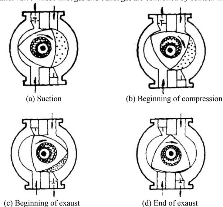
**Figure 1:** The working principle of Wankel compressor
