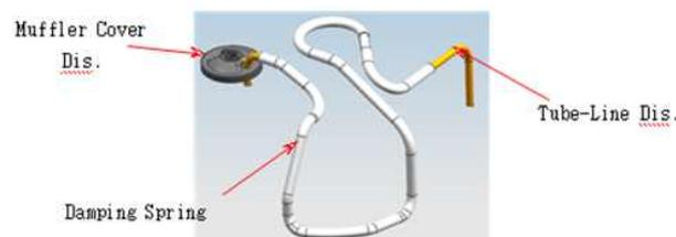
Figure 4 : Structure of LDT (Line Discharge Tube)
