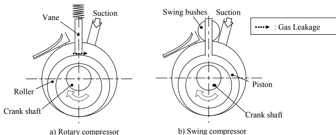
**Figure 1:** Mechanisms for swing compressor and rotary compressor
