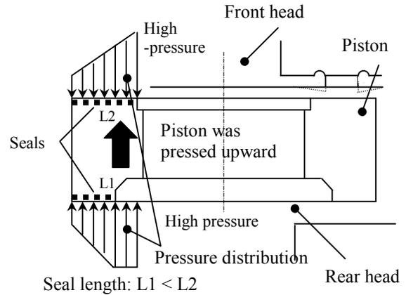
Figure 12: Shape of original piston
