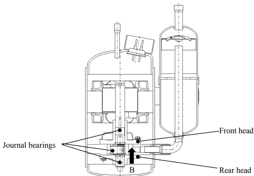
**Figure 10:** Section drawing
