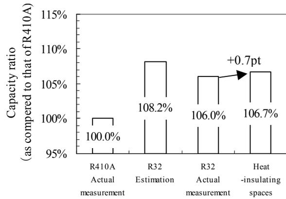
**Figure 5:** Heat-insulating effect
