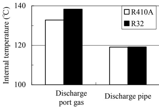
Figure 13: Internal temperature
