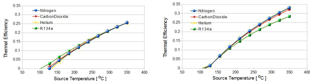
**Figure 2:** (Left) Thermal efficiency of regenerative Brayton cycle vs source temperature for various working fluids. (Right) Thermal efficiency of LFEC utilizing Therminol-66 vs source temperature for various working fluids.
