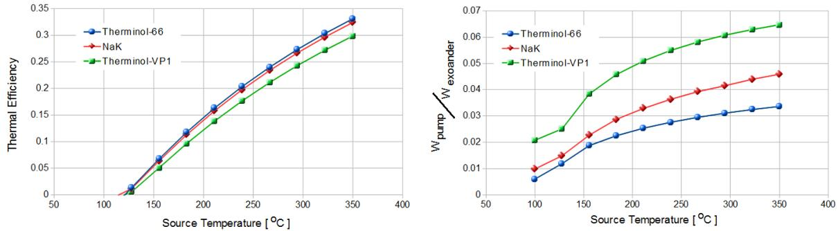
**Figure 3:** LFEC thermal efficiency (left) and relative pumping losses (right) for various flooding liquids
