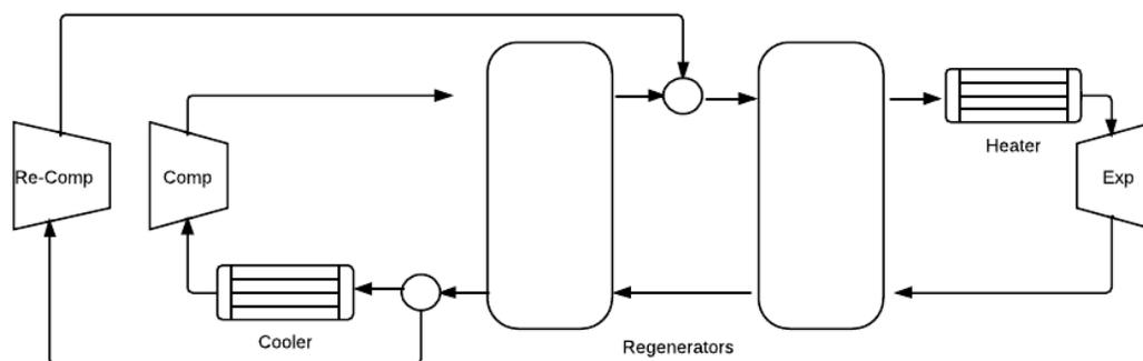
**Figure 7:** Recompression Brayton cycle. Two regenerators and a recompression stage are used to improve overall regenerator effectiveness and cycle thermal efficiency.
