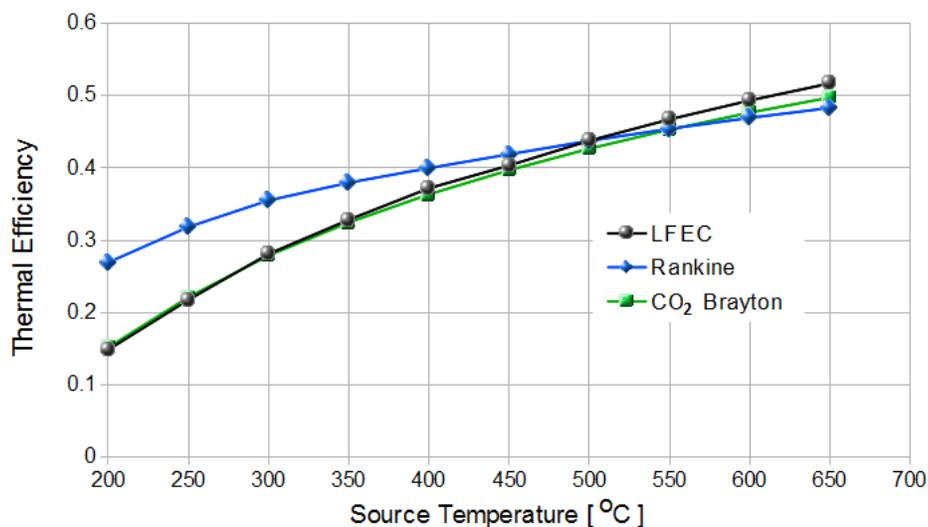
**Figure 8:** Comparison of LFEC to other cycles of interest to CSP systems
