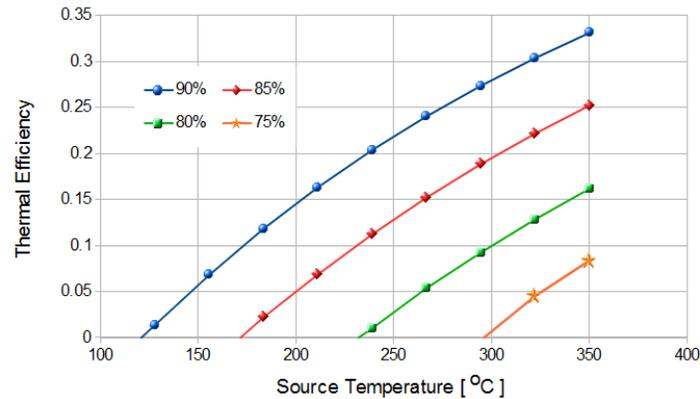
**Figure 5:** Thermal efficiency versus source temperature for multiple component efficiencies
