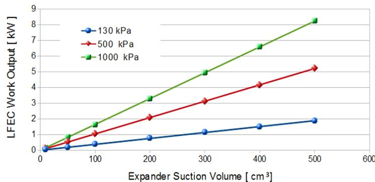
**Figure 4:** The work output of the LFEC using Therminol-66 for various expander suction volumes and multiple low side pressures. The expander is operating at a speed of 60 Hz.
