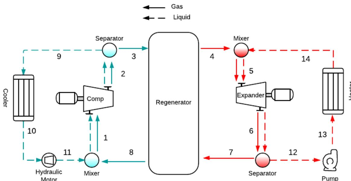
**Figure 1:** Liquid-Flooded Ericsson Cycle schematic
