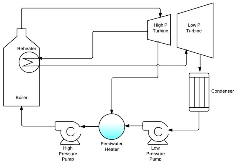
**Figure 6:** A Rankine cycle with 1 stage reheat and an open feedwater heater.
