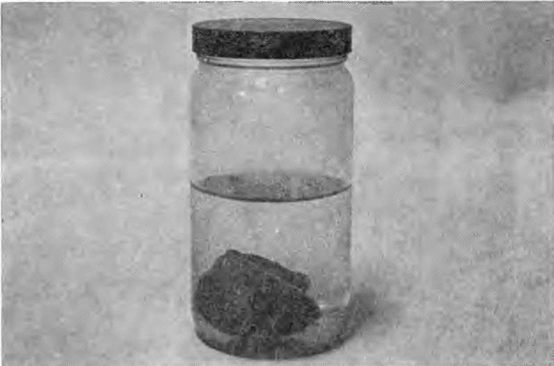
**Fig. 12. Paoli 3 Shale After 24 Hours of Immersion in Water.**
