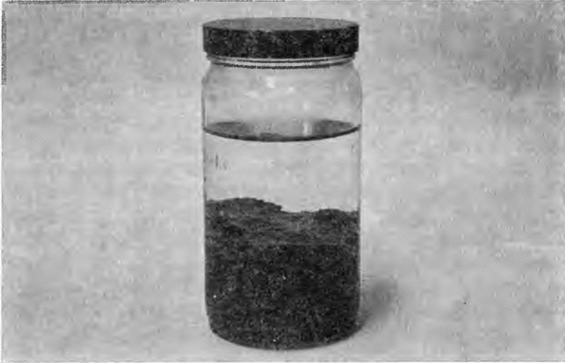
**Fig. 11. Cannelton Shale After 15 Minutes of Immersion in Water.**
