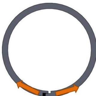
**Figure 3:** Tip seal with abutment joint
