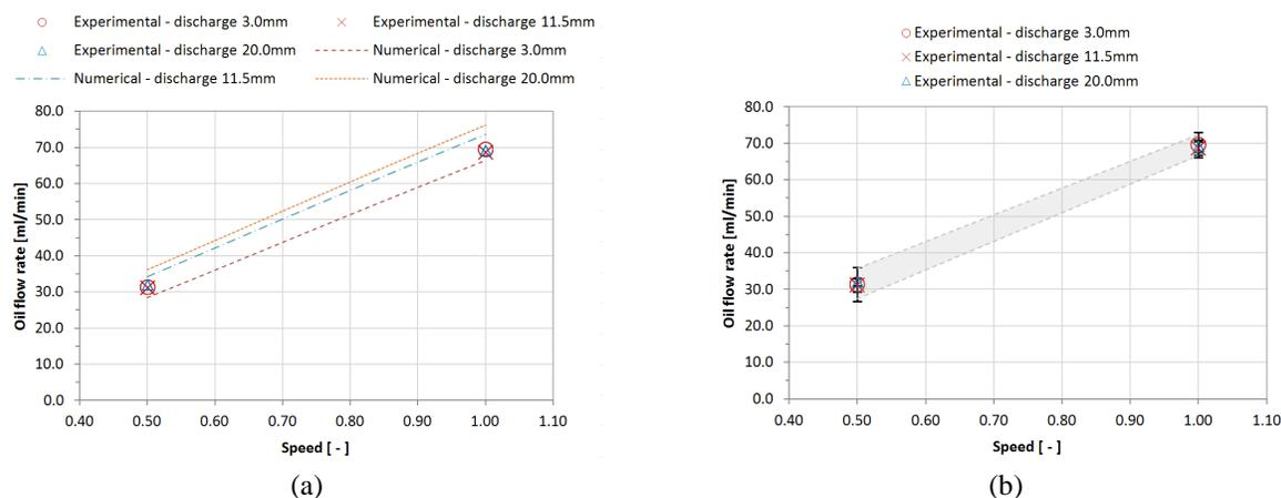
**Figure 4:** Oil flow rate over dimensionless rotation and discharge height: (a) experimental and numerical results; b) experimental uncertainties and interval of confidence for oil flow rate varying with rotation and immersion.
