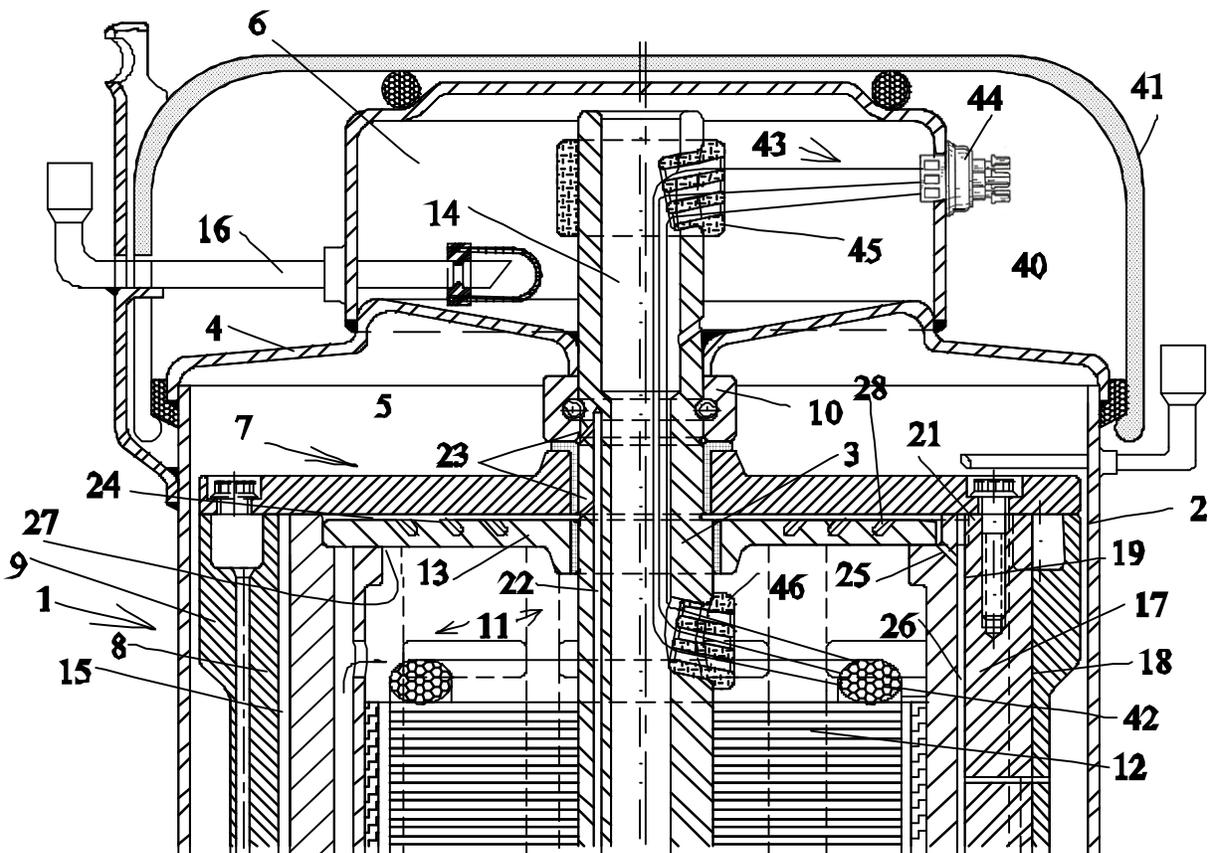
**Figure 2:** A side sectional view of a revolving piston compressor with the stationary crankshaft, (Dreiman, ,2013)
