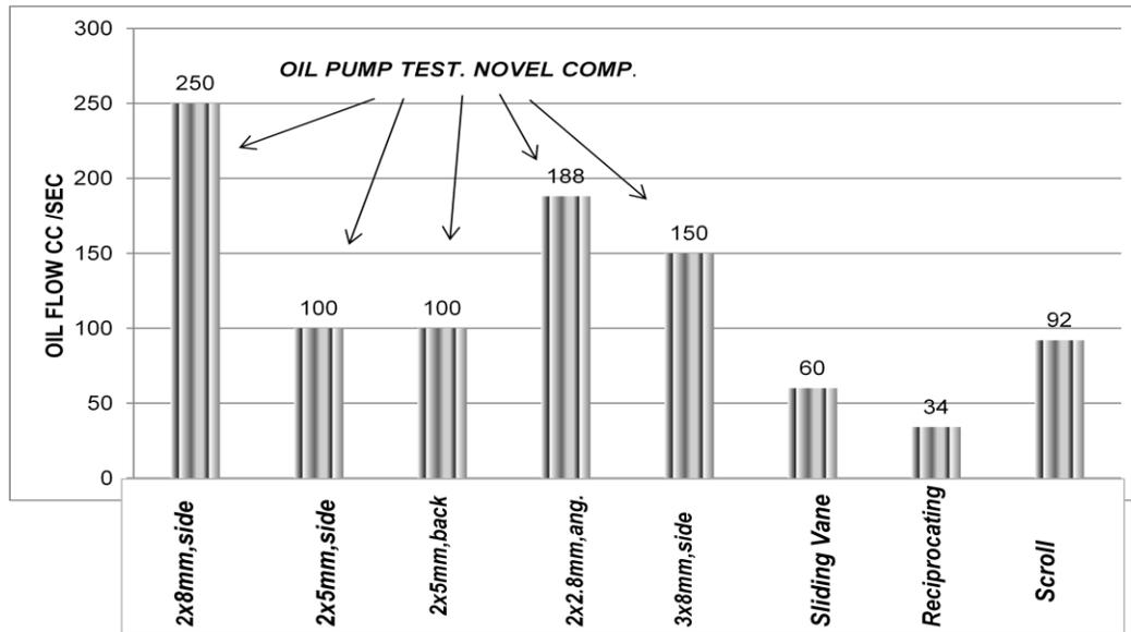
**Figure 4:** The oil flow test results of the pump with variety of inlet port diameters and positions
