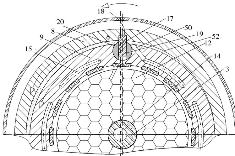
**Figure 3:** A horizontal cross-sectional view of the revolving piston rotary compressor, (Dreiman, 2013)
