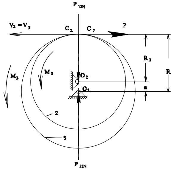
**Figure 1:** Schematic view of the rotor block (cylinder 2) and revolving piston (cylinder 3) coupling
