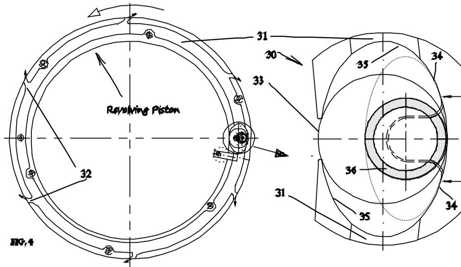
**Figure 5:** Top view of the revolving piston with the discharge nozzles and enlarged view of the valve, (Dreiman , 2013)
