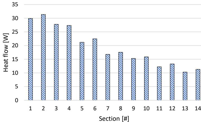
**Figure 7:** Heat flow per section for an inner tube temperature of 35 °C
