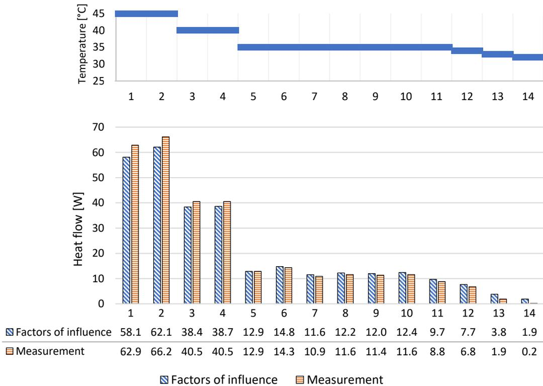
Figure 11: Inner tube temperature profile and heat flows for the second verification case
