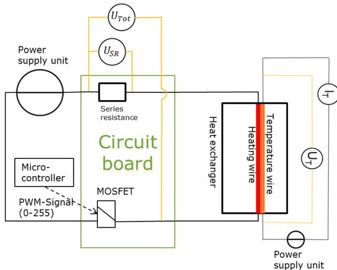
**Figure 4:** Measurement method
