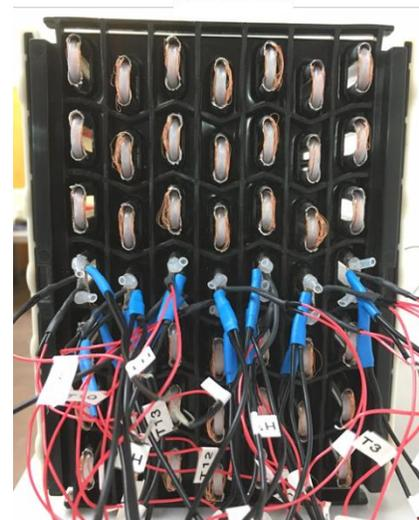
**Figure 3:** Wiring of the seven-row-wing-tube heat exchanger
