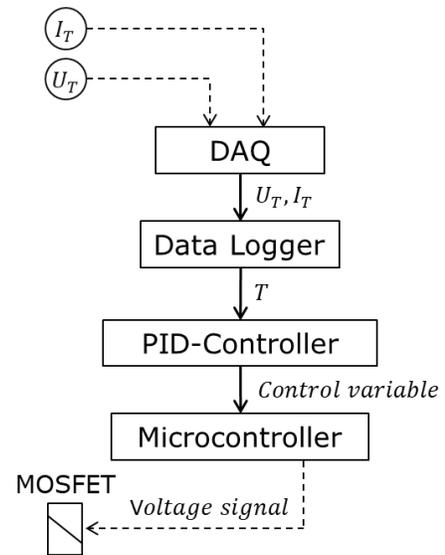
**Figure 5:** Control mechanism
