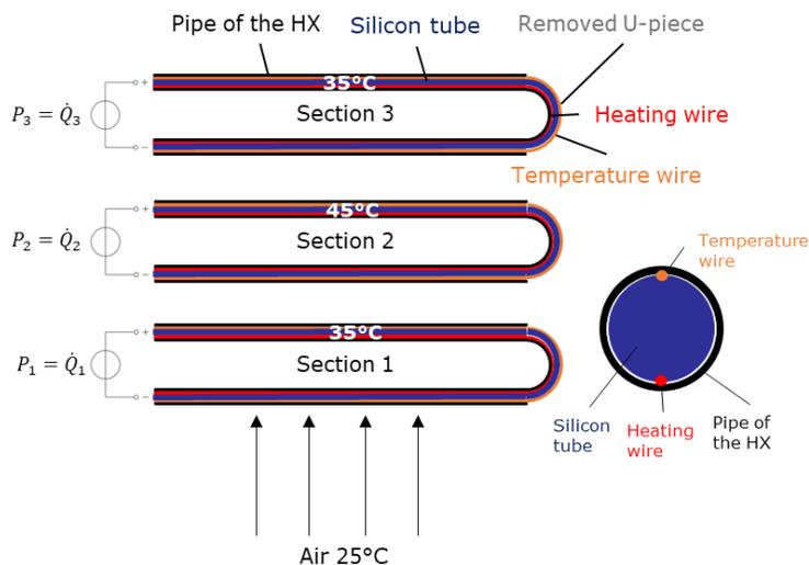
**Figure 2:** Schema of the measurement concept
