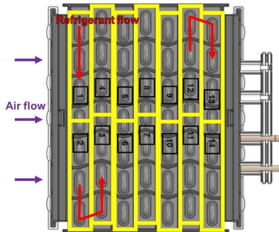
**Figure 1:** Spatial distribution of the heat exchanger
