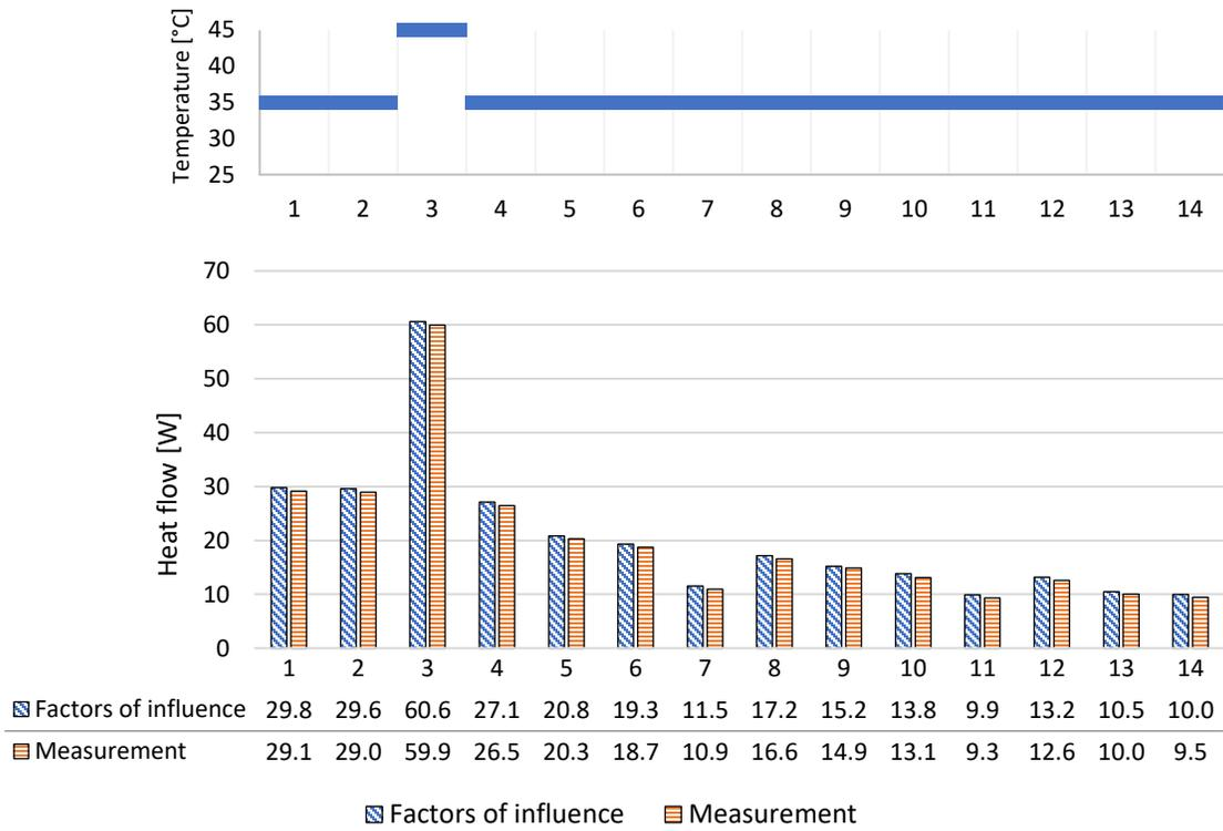
Figure 10: Inner tube temperature profile and heat flows for the first verification case
