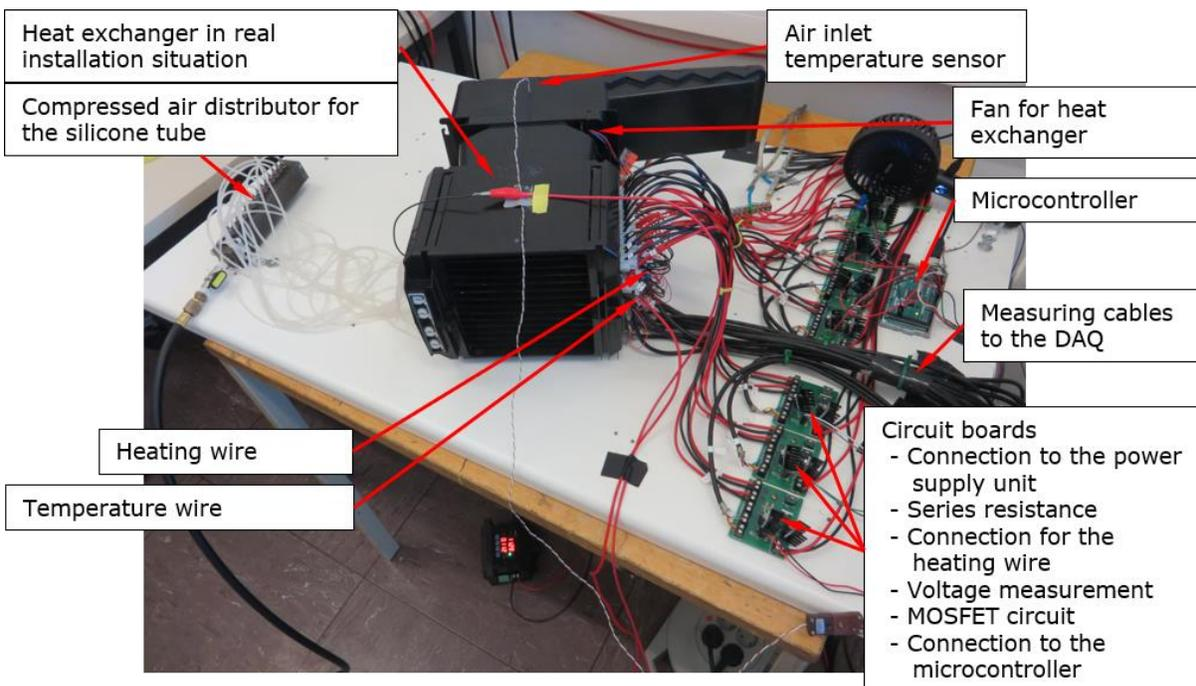
**Figure 6:** Measurement setup
