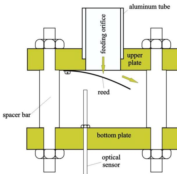
**Figure 2:** Test section
