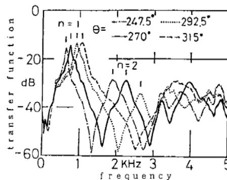
Figure 6: acoustic characteristic of discharge cavity of cylinder
