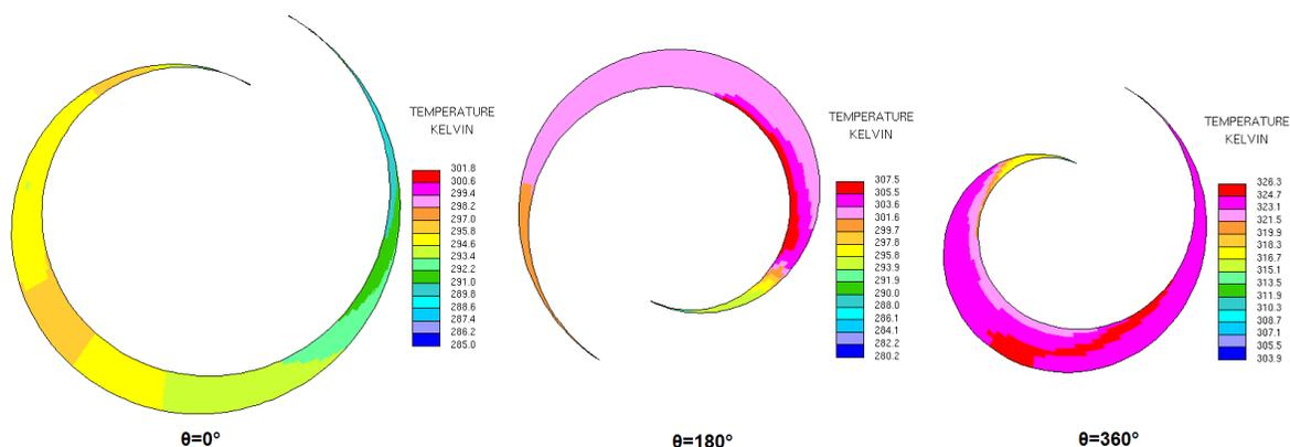
Figure 8: Temperature of the working chamber
