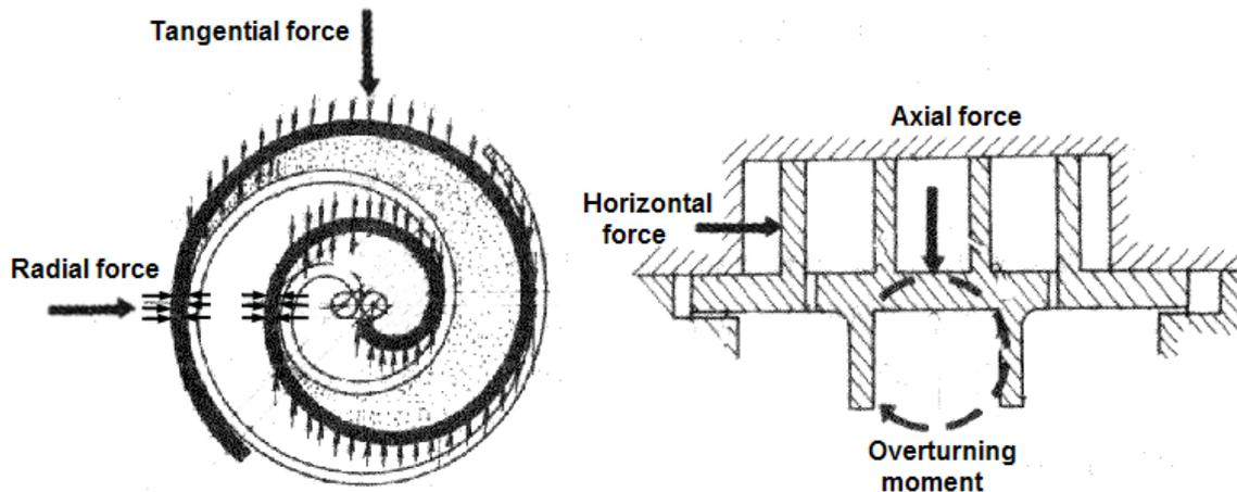
Figure 9: Illustration of gas forces on orbiting scroll
