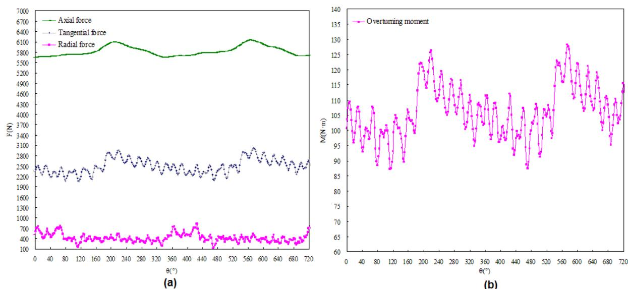
**Figure 10:** Gas forces and moment: (a) axial, radial and tangential force, (b) overturning moment
