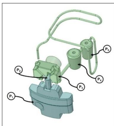
**Figure 6:** Pressure sensor positions.
