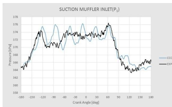
**Figure 10:** Suction Muffler Inlet results.
