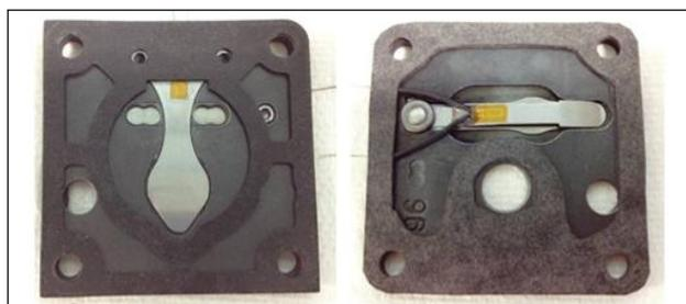
**Figure 8:** Strain gage bonded in the suction and discharge valve retainer.
