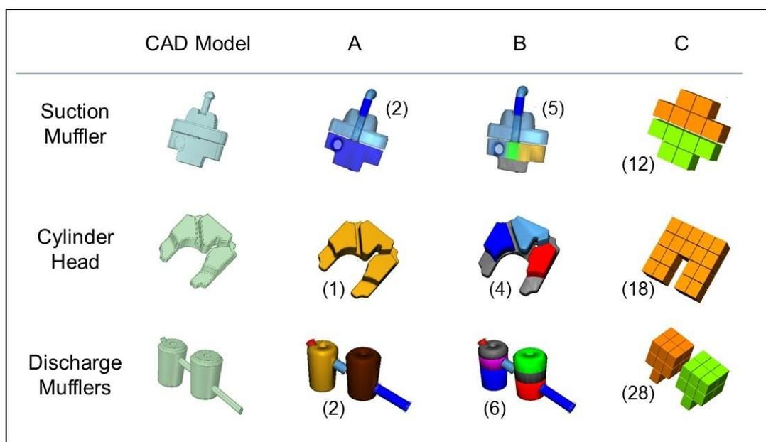
Figure 1: 3D components and their discretization levels.
