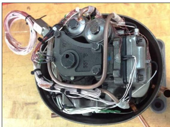
**Figure 7:** Overview compressor instrumented.
