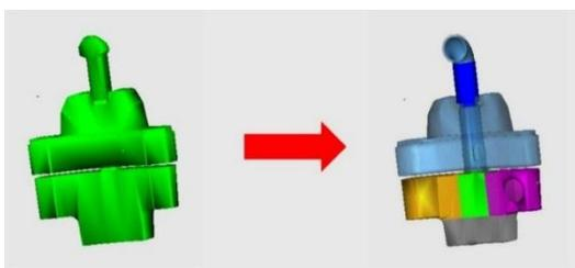
Figure 5: GT-Suite conversion from raw CAD to discretized volumes.
