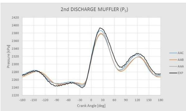
**Figure 17:** Second Discharge Muffler results
