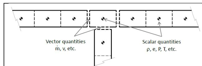
**Figure 2:** 1D flow volumes discretized into a staggered grid.
