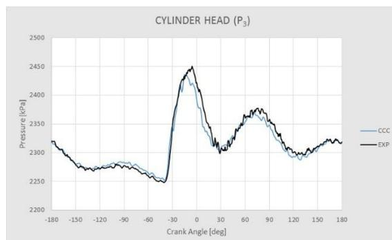
**Figure 14:** Cylinder Head pressure results.
