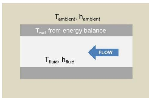
Figure 3: Schematic of Pipe thermal solution method.
