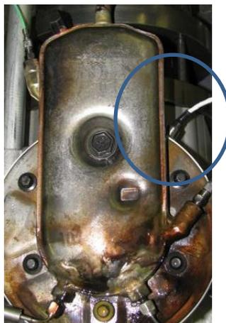
Figure 3. Pressure transducers mounted to suction plenum.
