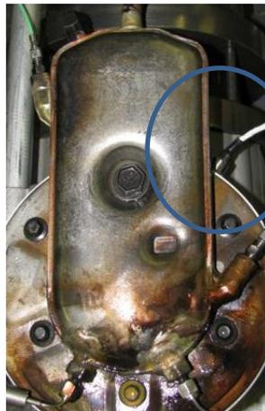
Figure 3. Pressure transducer mounted to suction plenum.
