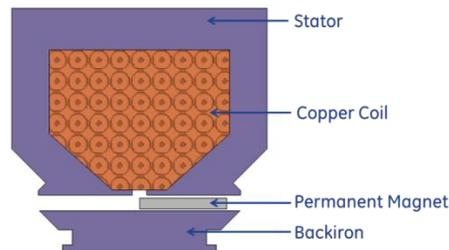
**Figure 4 Layout of Motor and stator**
