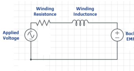
**Figure 5** Layout of RLC circuit of motor
