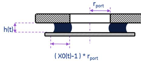
**Figure 3: Oil film between the valve seat and reed causes stiction**
