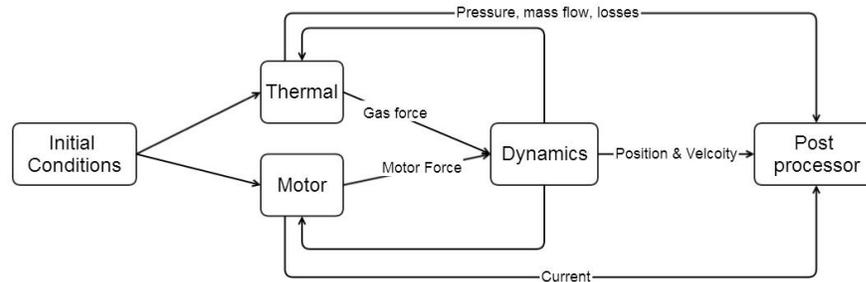
Figure 2: Simulation Block Diagram
