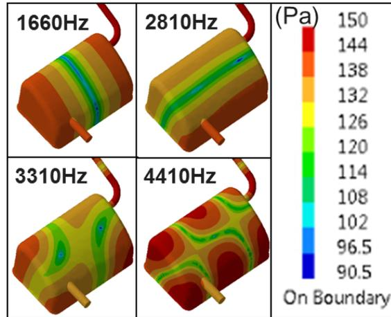
Figure 12: Pressure distribution of expansion chamber at first four acoustic modes of muffler
