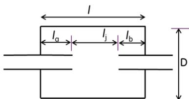
**Figure 10:** Schematic diagram of EIEO muffler
