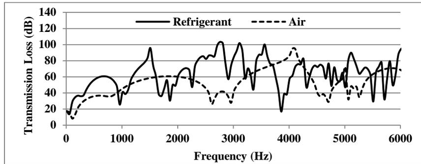
Figure 14: Transmission loss with refrigerant and air as medium
