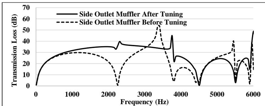
Figure 13: Transmission loss improvement of a tuned side outlet muffler
