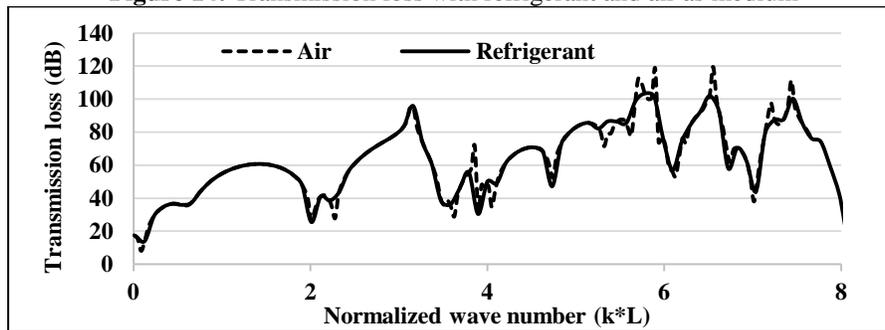
Figure 15: Transmission loss with refrigerant and air as medium plotted as function of normalized wave number
