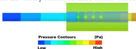
**Figure 8:** Pressure contours for EIEO muffler with perforated bridge
