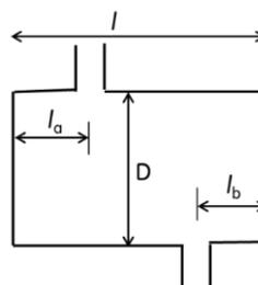
**Figure 11:** Schematic diagram of SISO muffler
