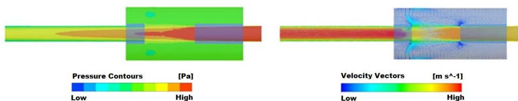
**Figures 7:** Pressure and velocity contours for EIEO muffler without perforated bridge
