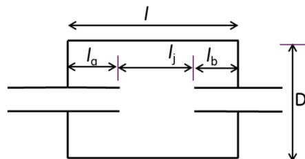
Figure 1: Schematic of extended inlet and extended outlet muffler (EIEO)
