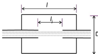
**Figure 9:** Schematic of EIEO muffler with flow jet passing without expansion
