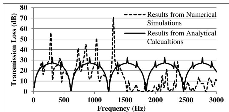
Figure 2: Comparison of analytical results with numerical simulation of an EIEO muffler
