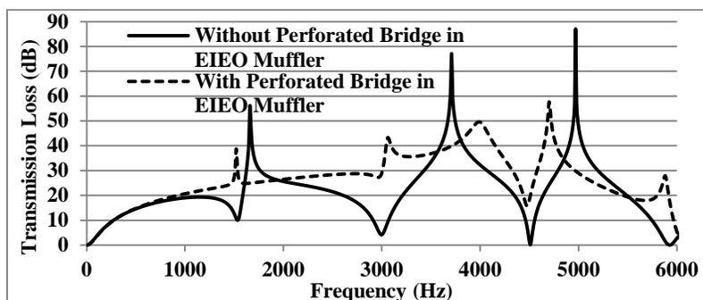
**Figure 6:** Transmission loss improvement of perforated bridge EIEO muffler
