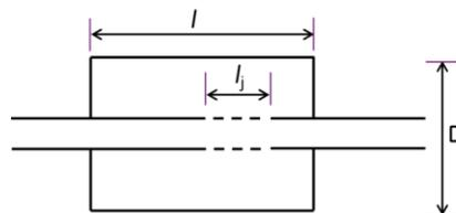
**Figure 5:** Schematic diagram of extended inlet and extended outlet muffler connected with perforated bridge
