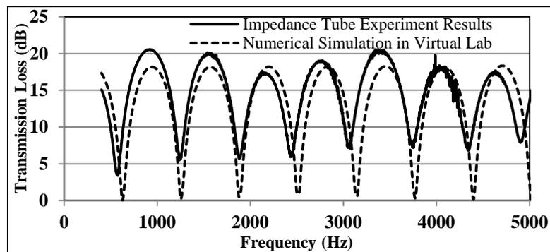
**Figure 4:** Comparison of numerical and experimental transmission loss curves
