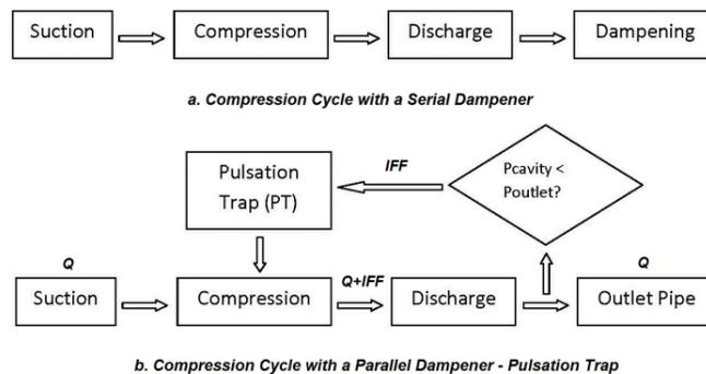
**Figure 9(a-b):** Comparison of a Shunt Pulsation Trap with the conventional serial configuration for UC mode
