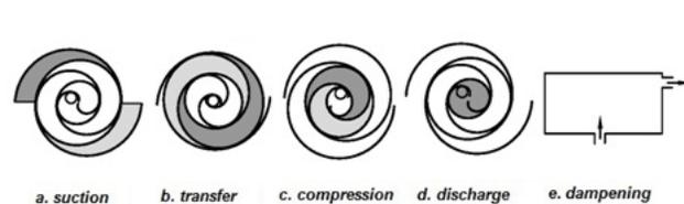
**Figure 5(a-e):** Conventional scroll compression cycle with a serial dampener at discharge
