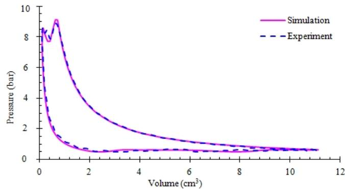
Figure 5: Pressure inside cylinder
