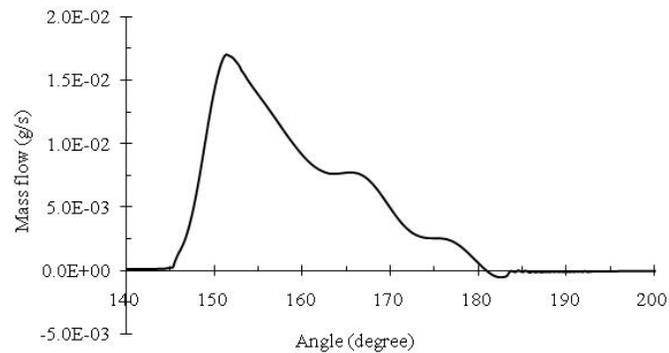
**Figure 8:** Mass flow rate through exhaust port
