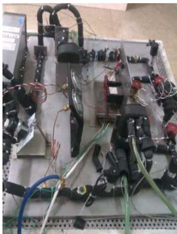
**Figure 1:** Experimental design of the test system for compressor performance
