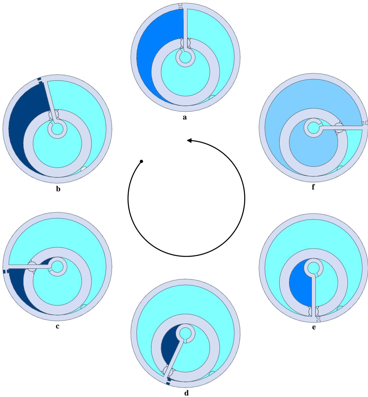
**Figure 4:** The working principle of CVEC
