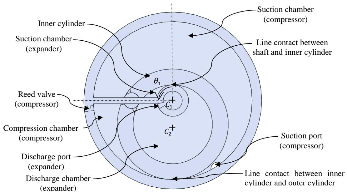
**Figure 2:** Front sectional view of CVEC
