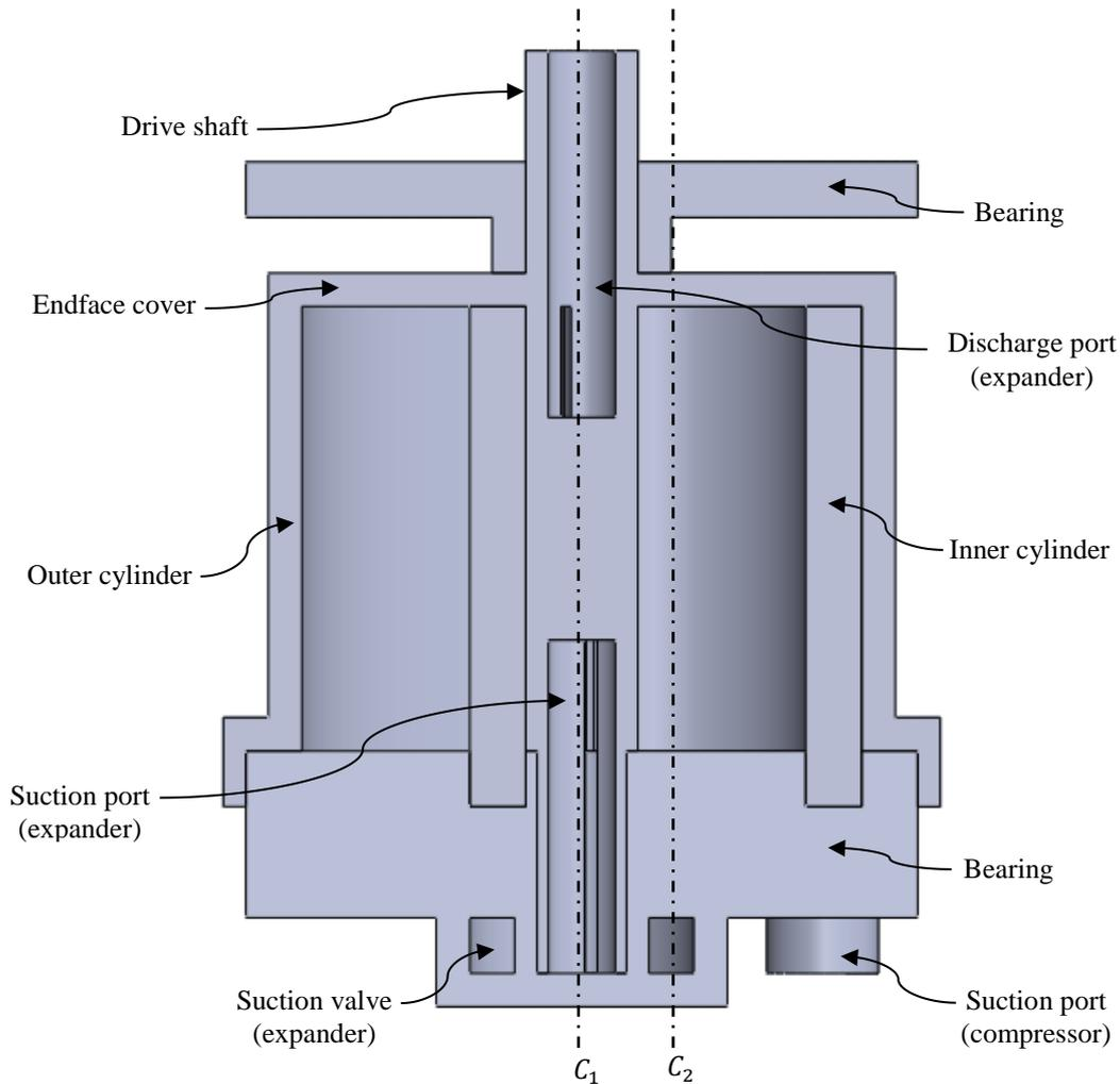
**Figure 3:** Side sectional view of cantilever type CVEC
