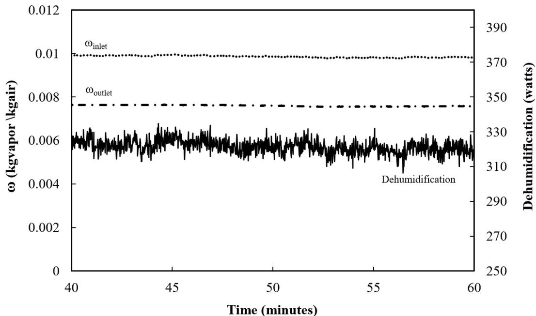
**Figure 5:** Steady-state experimental measurement of dehumidification capacity and air specific humidity ( $\omega$ )
