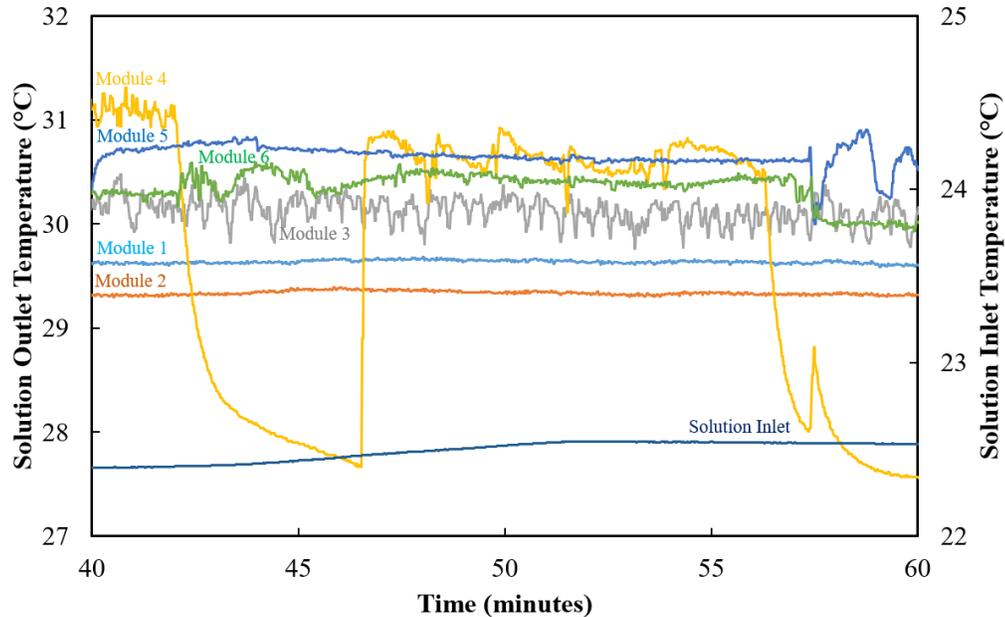
**Figure 6:** Steady-state experimental measurements of absorber inlet and outlet solution temperature for the six modules running in parallel. One module (module 4) appeared to have intermittent solution flow
