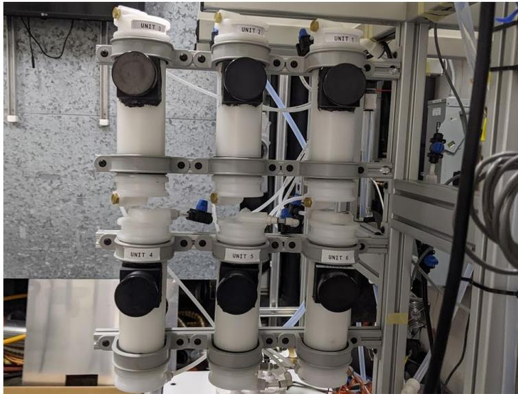
**Figure 2:** Six membrane contactors in a parallel configuration. The black holes are the air inlets, shown capped.
