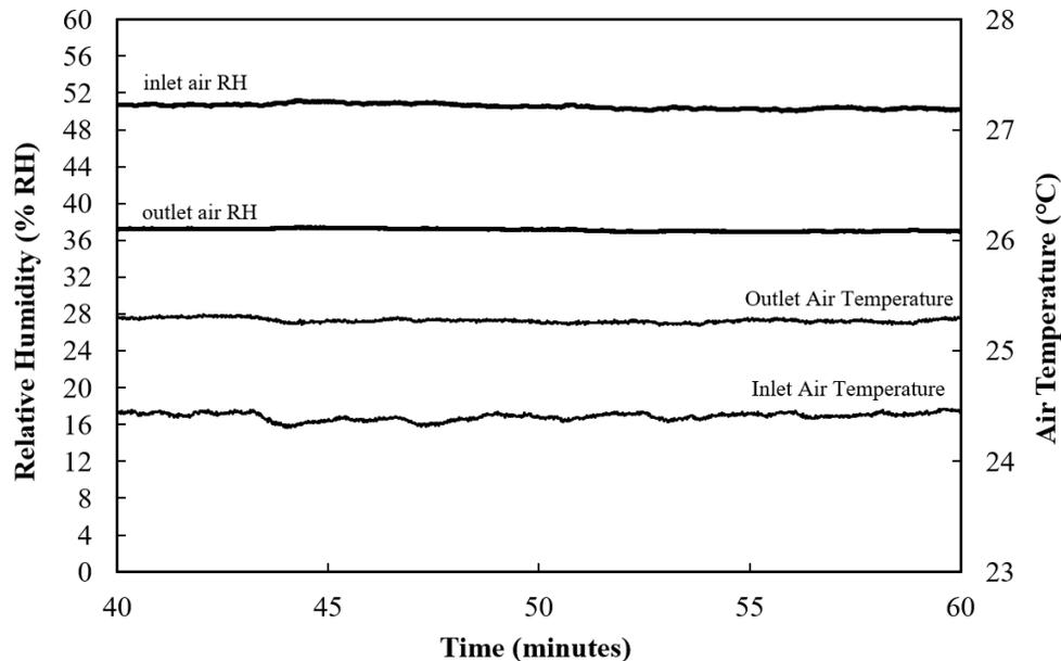
**Figure 4:** Steady-state experimental measurements of ambient air inlet and outlet conditions
