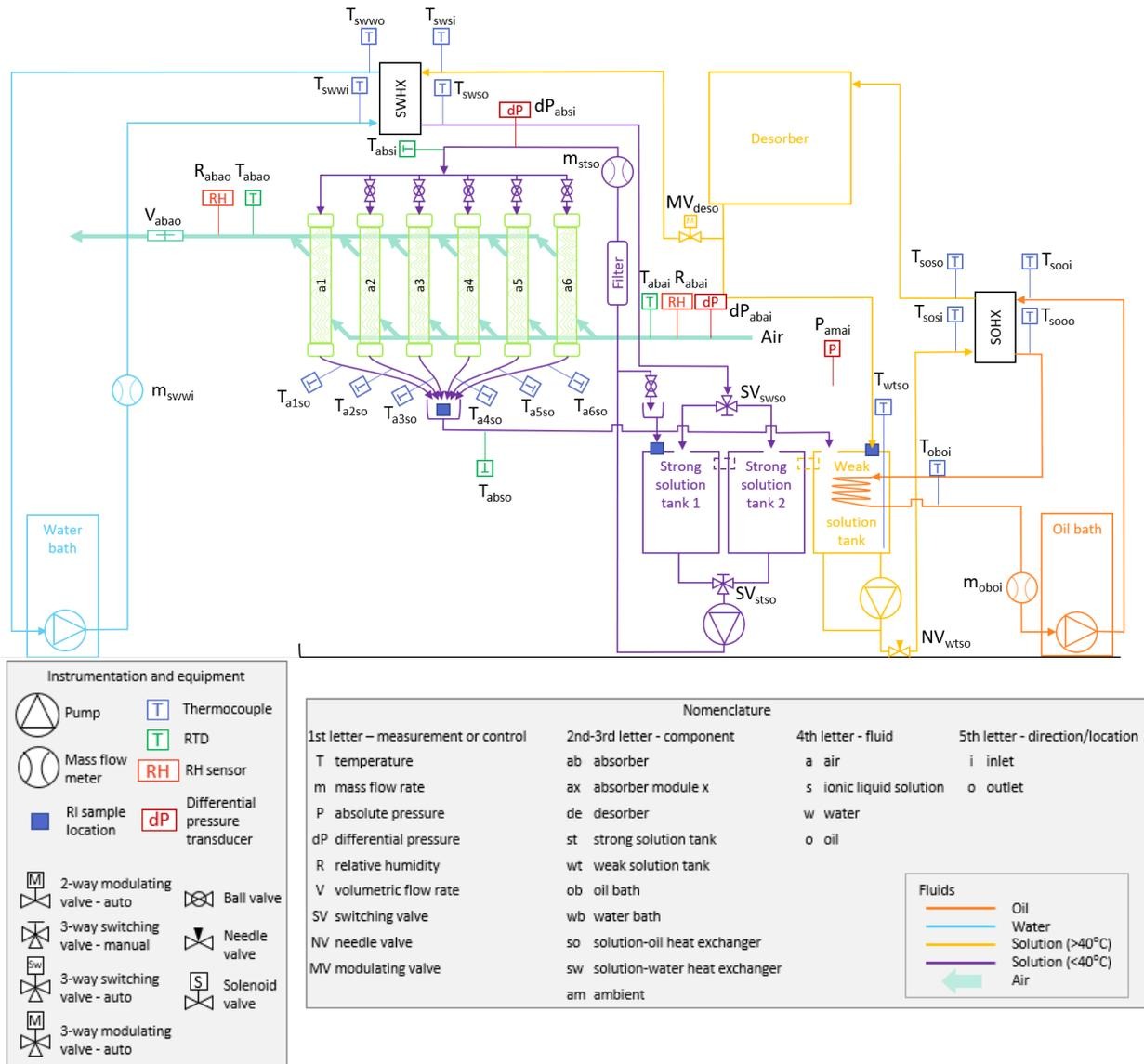
**Figure 3:** Process and instrumentation diagram of the air dehumidification unit. Naming convention: 1<sup>st</sup> letter represents the measured property or control unit, 2<sup>nd</sup> and 3<sup>rd</sup> letter represent the system component, 3<sup>rd</sup> letter represent the type of fluid, and 4<sup>th</sup> letter represent the direction of the flow.
