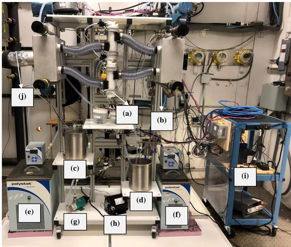
**Figure 1:** Experimental set-up for a novel air dehumidification module where (a) membrane fiber bundle module, (b) inlet air header, (c) strong solution tank, (d) weak solution tank, (e) cooling water bath, (f) heating oil bath, (g) weak solution pump, (h) strong solution pump, and (i) data acquisition and control unit, and (j) air flow measurement station
