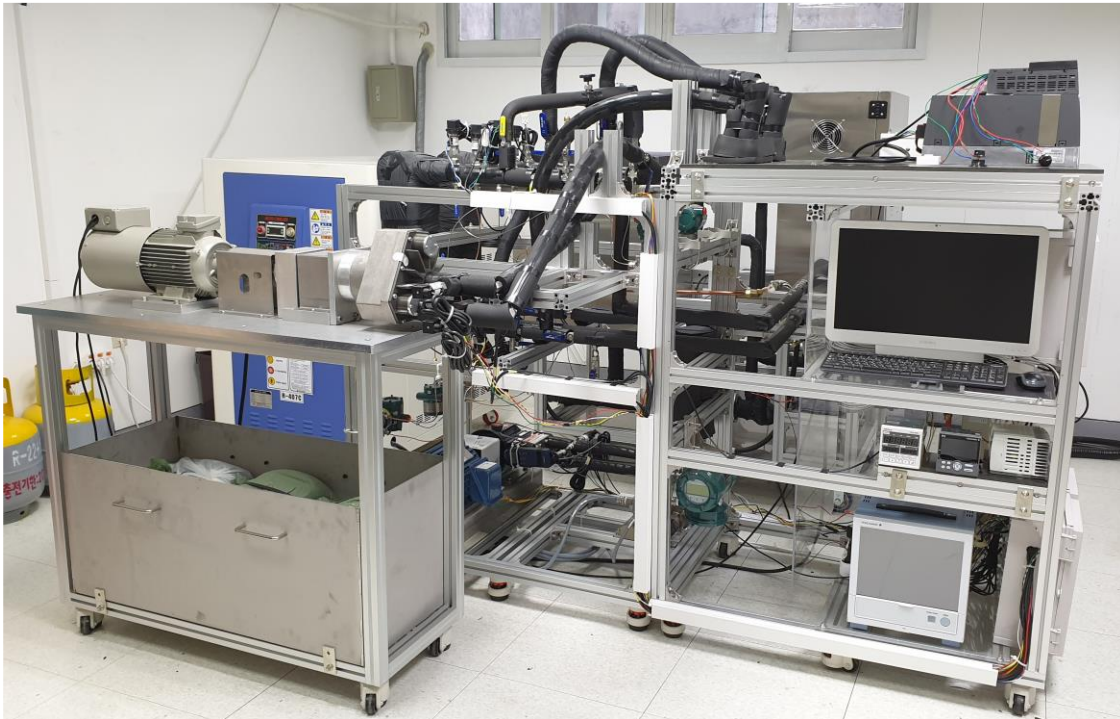
Figure 1: Photograph of the 1 kW lab-scale ORC testbed
