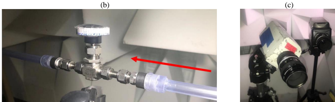
Figure 2. Experimental setup and system schematic (a) system schematic (b) horizontal transparent tubes (c) high-speed cameras (Phantom V4.2)
