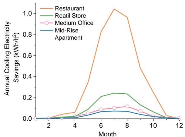
**Figure 7:** Normalized monthly cooling electricity savings profile for several different building types located in Houston, Texas, generated using EnergyPlus building simulations.
