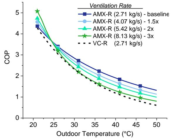
**Figure 5:** System COP of the AMX-R for various ventilation mass flowrates ( $\dot{m}_v$ ) compared to the VC-R system operating at the baseline ventilation rate specified by ASHRAE 62.1 (from EnergyPlus).
