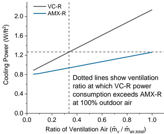
**Figure 4:** Cooling power consumption for the AMX-R and VC-R systems as a function of the ratio of the ventilation air to total air mass flowrates for the conditions specified in Table 1.
