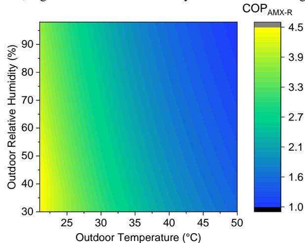
**Figure 2:** System COP of the AMX-R configuration as a function of the outdoor air temperature and humidity, presented for outdoor air conditions ranging between 20-50 °C and 30-100% relative humidity.
