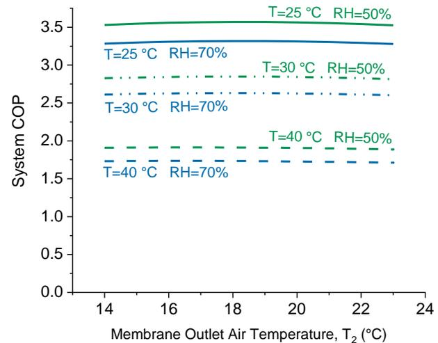
**Figure 3:** AMX-R system COP as a function of the membrane module outlet air temperature for several ambient temperature and humidity conditions. This figure shows the optimal range of module outlet air temperatures.
