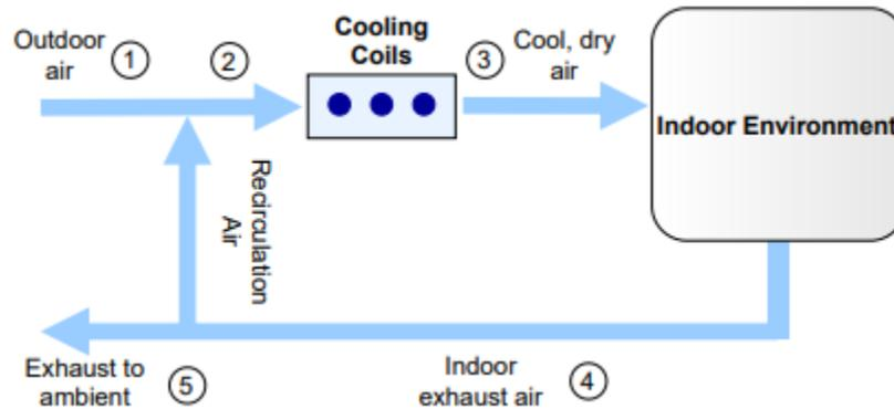
**Figure A1:** Conventional vapor compression system that features both air recirculation and mechanical ventilation (VC-R) used as the baseline system for comparison in this work.
