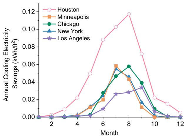
**Figure 6:** Normalized monthly cooling electricity savings profile for a “Medium Office Building” in five major US cities spanning numerous climate zones, generated using EnergyPlus building simulations.
