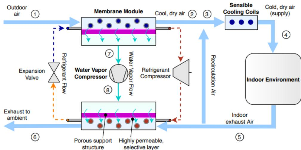
**Figure 1:** System schematic showing the novel Active Membrane Energy Exchanger device incorporated into a system with air recirculation and mechanical ventilation (AMX-R). The Active Membrane Energy Exchanger portion (two membrane modules and the integrated cooling cycle) provides all of the dehumidification required to meet the desired supply humidity and provides some sensible cooling. The mixed air is then sent to the separate sensible cooling coils.
