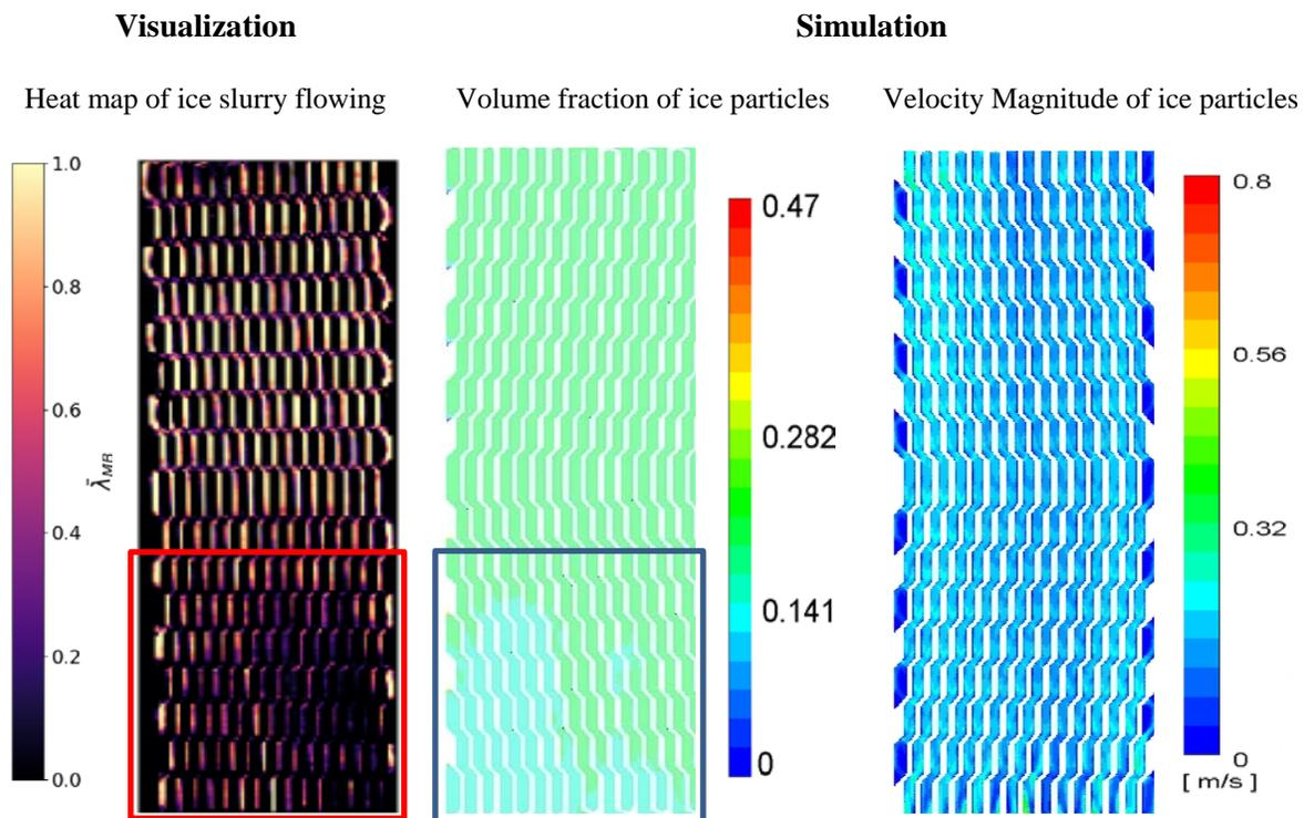
**Figure 6:** Comparison between the visualization profiles with simulation profiles for ice particles
