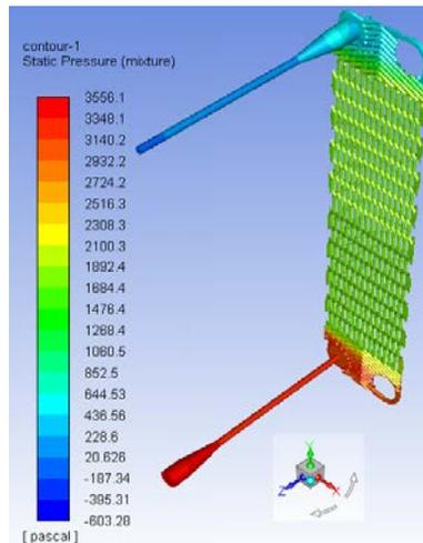
**Figure 5:** Static pressure of the mixture flow at V=1.86 l/min and ice volume fraction 20% inside the special plate heat exchanger geometry of TTZ Company
