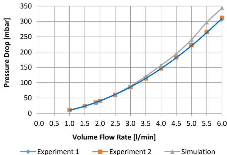
**Figure 3:** Pressure losses of the single-phase potassium formate-water flow as a function of the inlet volume flow in the special plate heat exchanger geometry of TTZ Company
