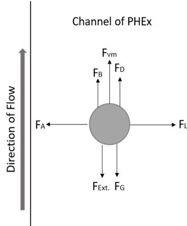
**Figure 2:** Forces acting on a particle through the channel of plate heat exchanger
