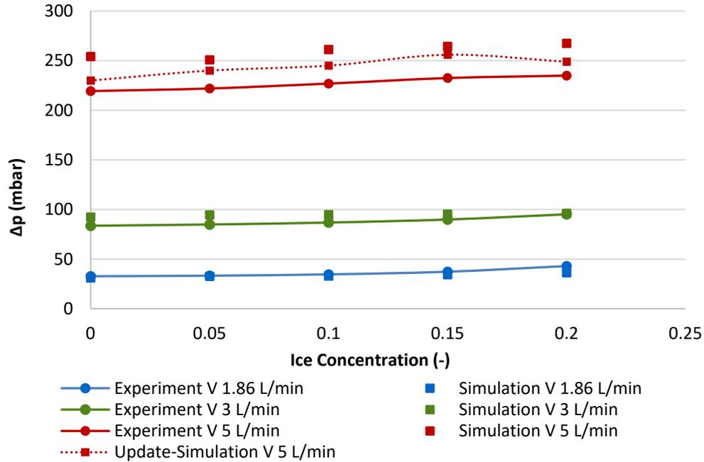
**Figure 4:** Validation of the pressure drop between experimental and simulation results of the special plate heat exchanger geometry of TTZ Company
