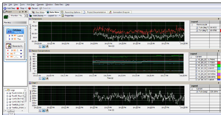
Figure 5: NI SignalExpress sample output display. Temperatures displayed in the upper graph. The middle graph displayed live CO 2 concentration data. The bottom graph displayed leak discharge pressure. A spike in discharge pressure indicates the starting time of the refrigerant leak.
