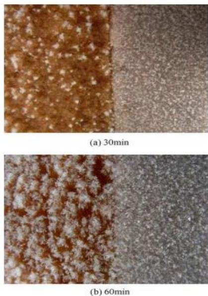
Fig. 7: Comparison of frost growth on the coated (left, thickness = 0.3 mm) and the uncoated (right) surfaces
