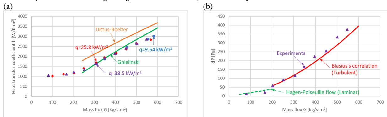
**Figure 4:** Comparison of the (a) heat transfer coefficient and (b) pressure drop of the liquid water inside smooth tubes with the correlations at different mass fluxes
