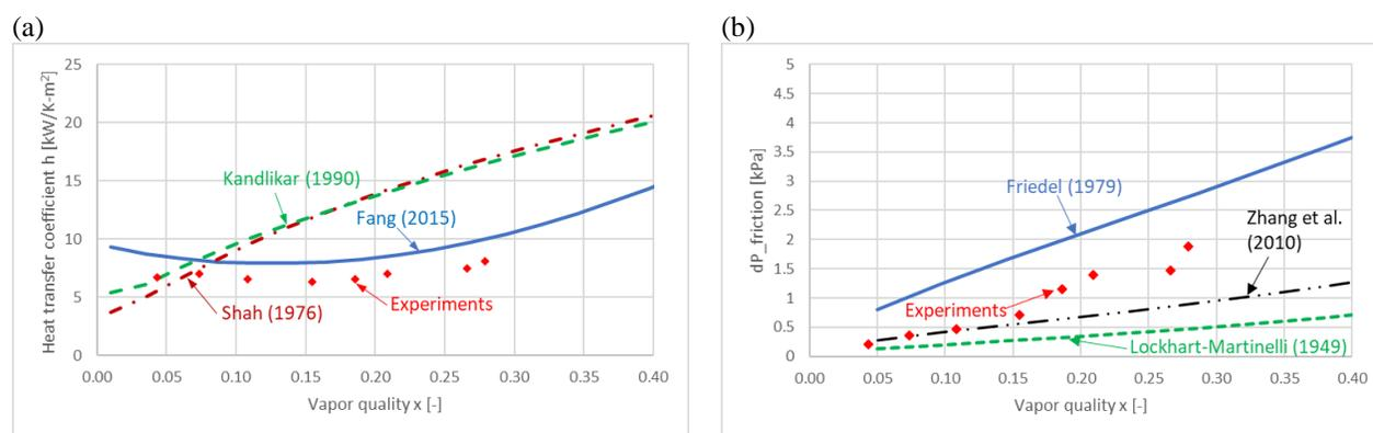
**Figure 5:** Comparison of the (a) heat transfer coefficient and (b) frictional pressure drop for the flow boiling of water inside smooth tubes with the correlations at various vapor qualities
