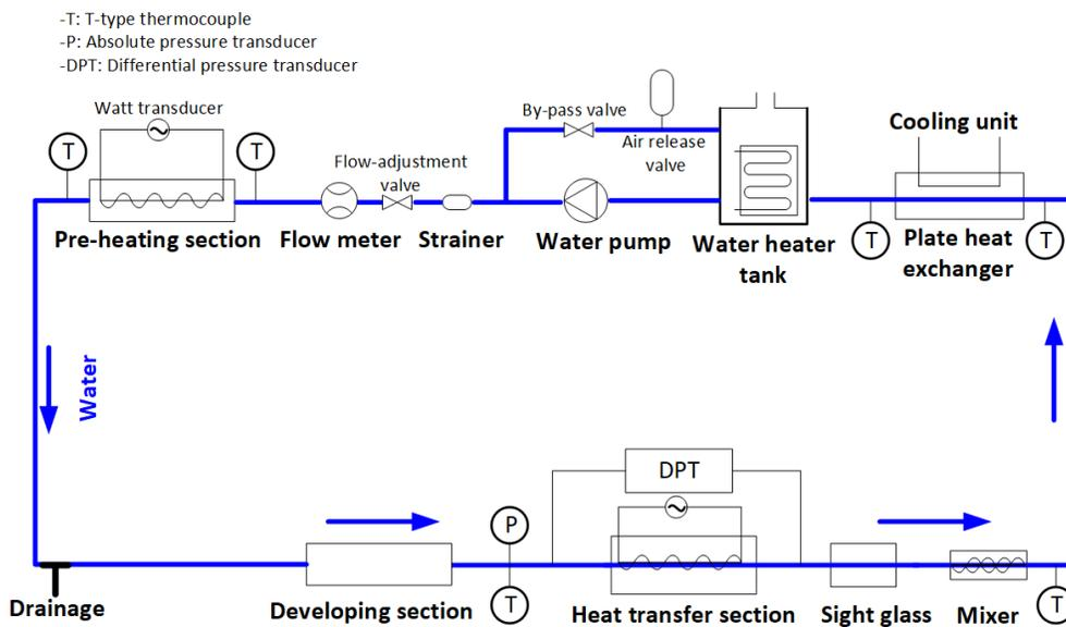
Figure 1: Schematic of test apparatus
