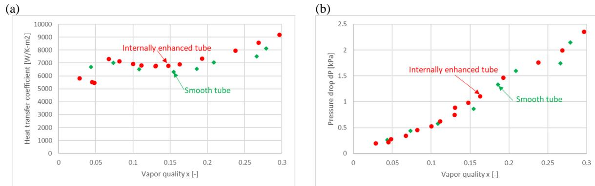
**Figure 9:** Comparison of (a) heat transfer coefficient and (b) total pressure drop of flow boiling of water in smooth and internally enhanced tube ( $G=80 \text{ kg/s-m}^2$ ,  $q=34 \text{ kW/m}^2$ )
