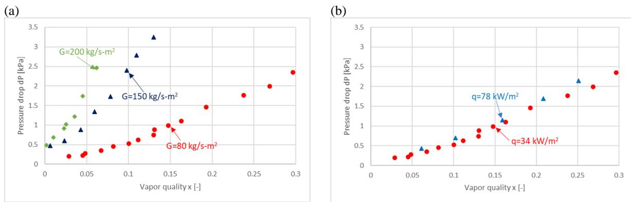
Figure 7: Effects of (a) mass flux and (b) heat flux on the total pressure drop of the flow boiling of water
