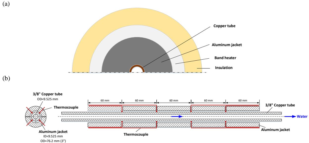
**Figure 2:** (a) Cross sectional view of the heat transfer test section and (b) locations of thermocouples
