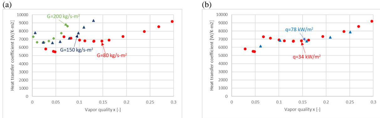
Figure 6: Effects of (a) mass flux and (b) heat flux on the heat transfer coefficient of the flow boiling of water
