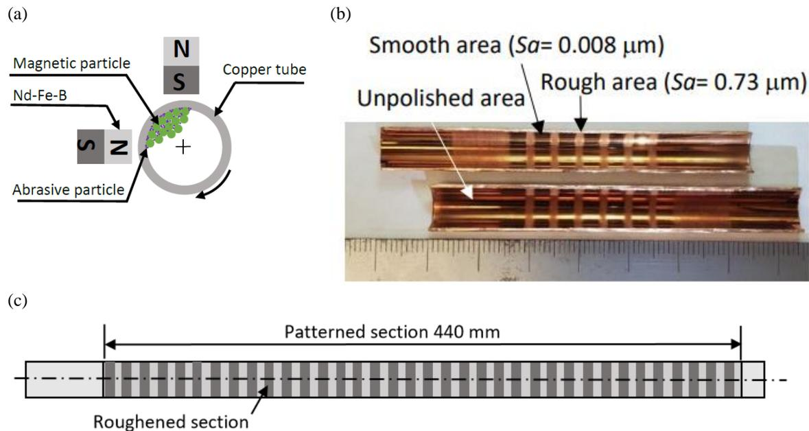
**Figure 3:** (a) Principle of MAF process, (b) representative polished surface of copper tube and (c) surface pattern of the sample tube
