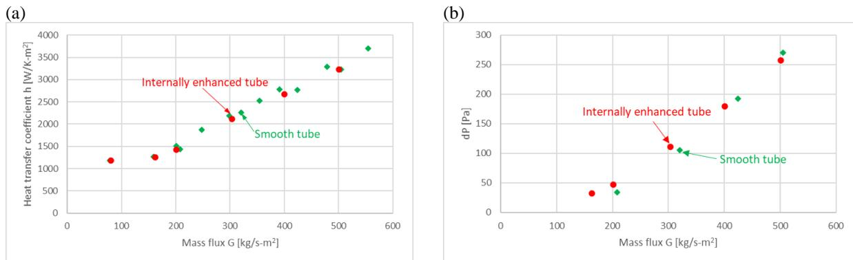
Figure 8: Comparison of (a) heat transfer coefficient and (b) total pressure drop of liquid water in smooth and internally enhanced tube ( $T=57^{\circ}\text{C}$ ,  $q=34\text{ kW/m}^2$ )
