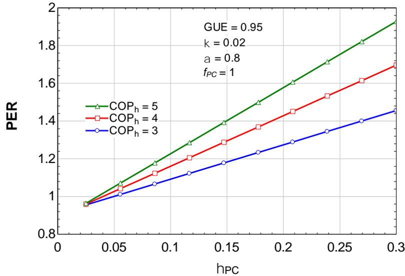
**Figure 5:** PER as a function of power cycle efficiency for a SPD-HP, with contours for various heat pump COP values.
