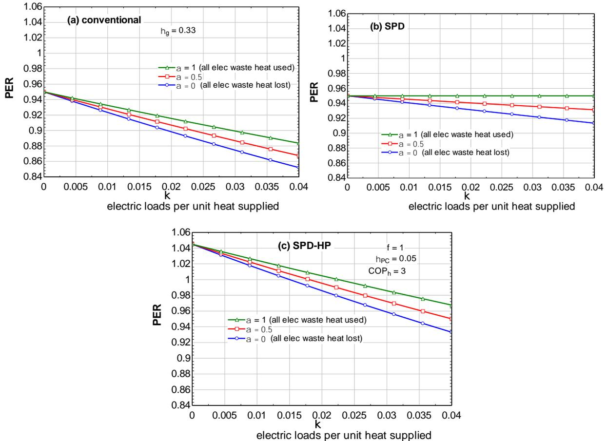
**Figure 4:** PER as a function of electric loads ( $\kappa$ ), with contours for various values of waste heat capture ( $\alpha$ ), for (a) conventional device, (b) self-powered device, and (c) self-powered device with heat pump.
