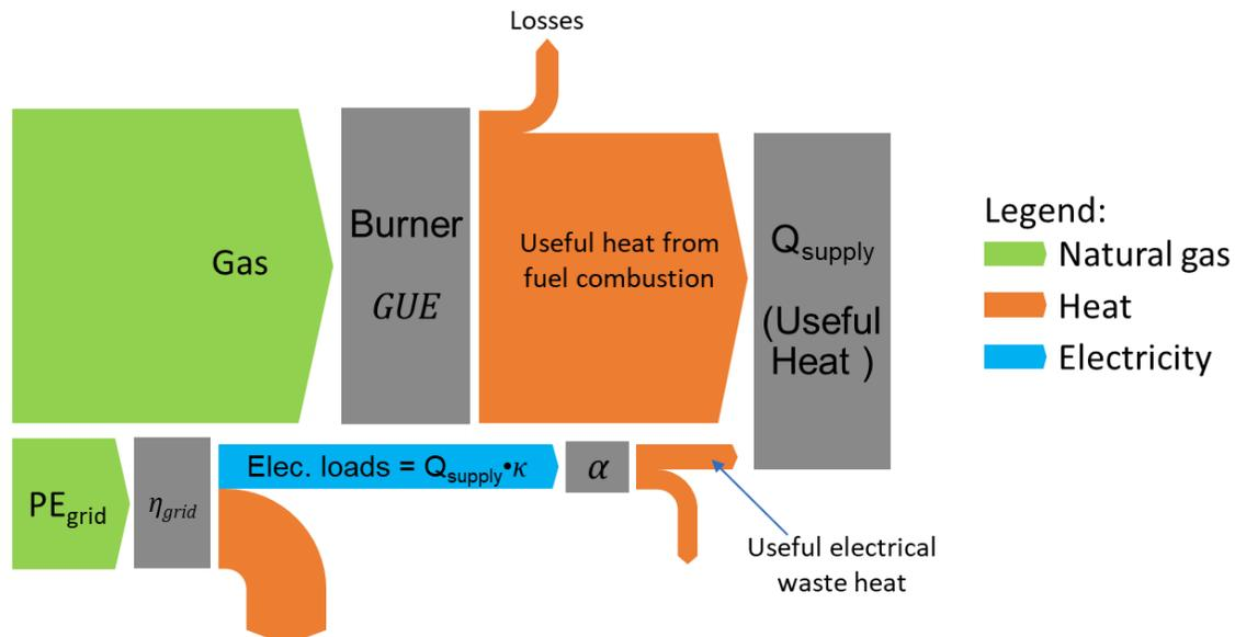
**Figure 1:** Sankey diagram of energy flows for a conventional heating device that draws electricity from the grid for electrical loads.
