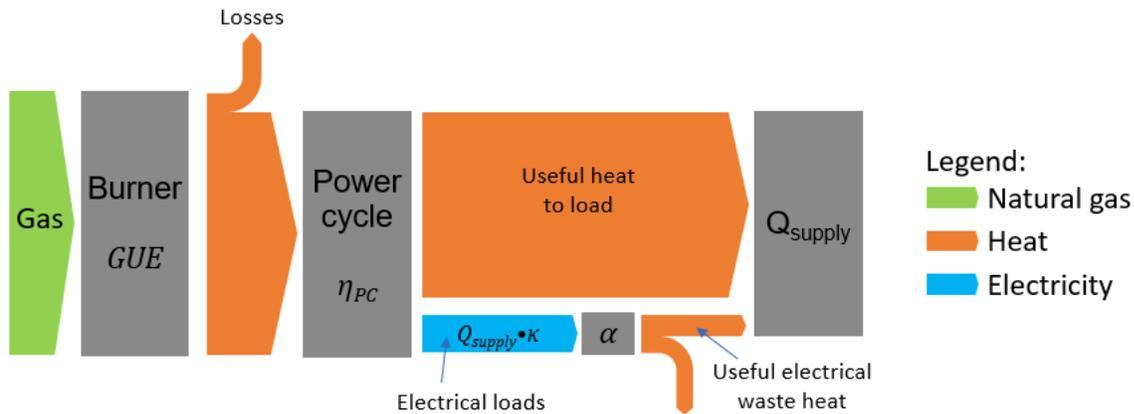
**Figure 2:** Sankey diagram of energy flows for a self-powered heating device.
